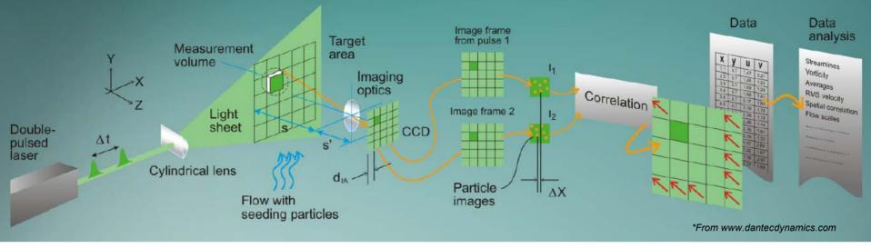
**Particle Image** Velocimetry (PIV) is a whole-flow-field Ο  $I_1$  $v = \frac{\Delta y}{\Delta t}$ visualization technique that  $\Delta t$ provides instantaneous velocity vector y  $I_2$ measurements in a 0 cross-section of a  $\mathcal{U}$ x = $\Delta t$ flow
