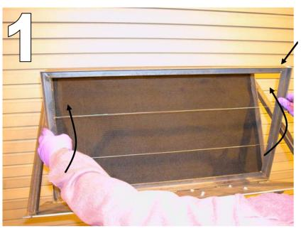
Roll the retainer frame in from the bottom to the top
