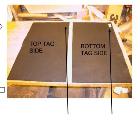
On the top blanket, cut edge is installed on the bottom of the frame. On the bottom blanket, the tag gets installed on the bottom of the frame.
