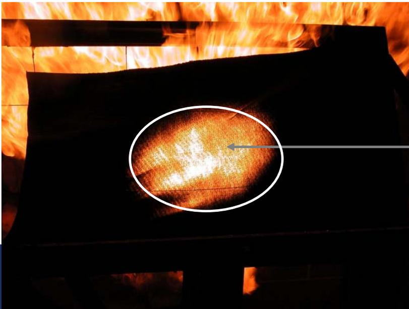
Material will typically shrink within 20 sec. from the top and the sides. The center portion, where the burnthrough is occurring, will not be affected by this. Sometimes, flashing will occur on the backside, but only lasts for a few seconds. This is acceptable.
