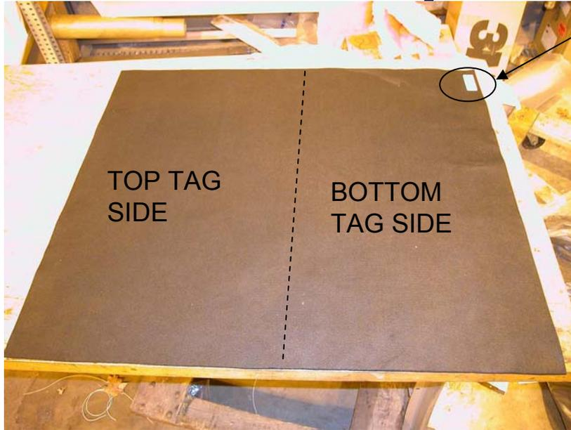
Tag indicates the "bottom" blanket, and also is the backside - not facing the flame.
