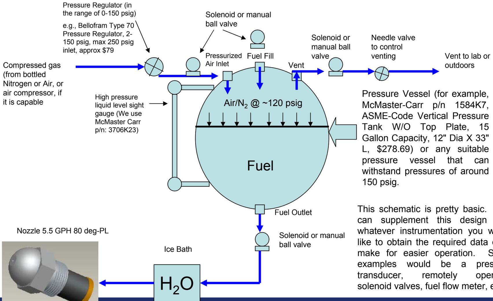
This schematic is pretty basic. You can supplement this design with whatever instrumentation you would like to obtain the required data or to make for easier operation. Some examples would be a pressure transducer, remotely operated solenoid valves, fuel flow meter, etc.
