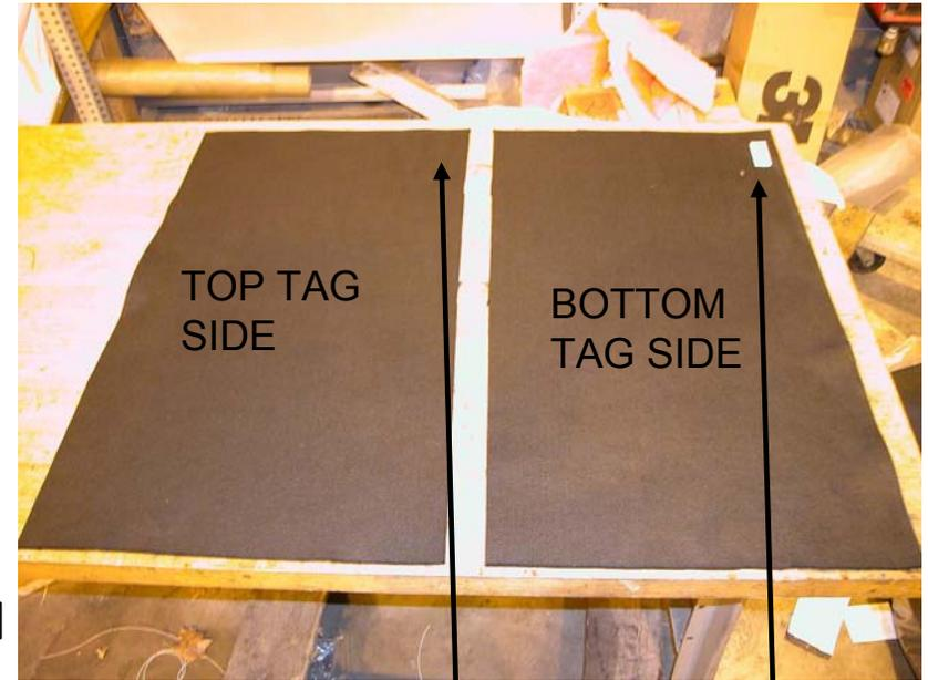
On the top blanket, cut edge is installed on the bottom of the frame. On the bottom blanket, the tag gets installed on the bottom of the frame.
