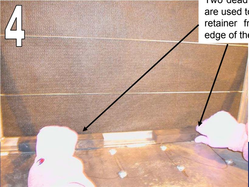
Two dead weights, about 5 lbs each, are used to put additional force on the retainer frame to keep the bottom edge of the blanket from shrinking up.
