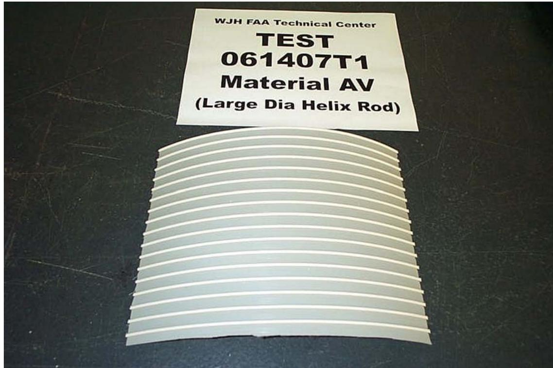
Example of a Material that Requires the Usage of the Special Condition Acceptance Criteria – Sample AV
