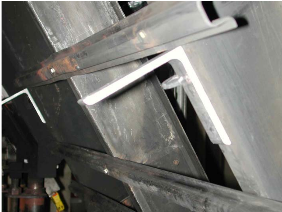
Figure 10. 4-inch Angle Clips Attached to Outer Formers
