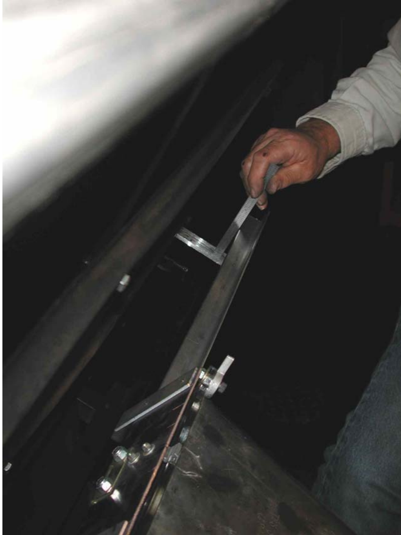
Figure 11. Measuring Vertical Distance to Centerline Using Long Angle on Faceplate
