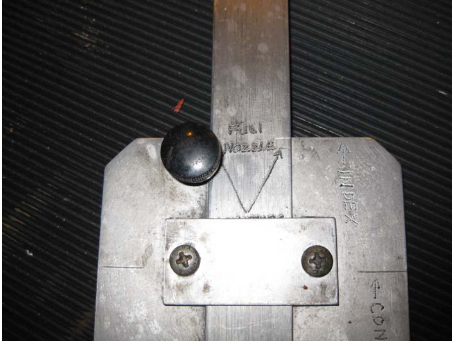
Figure 4. Scribe Mark for Fuel Nozzle Depth
