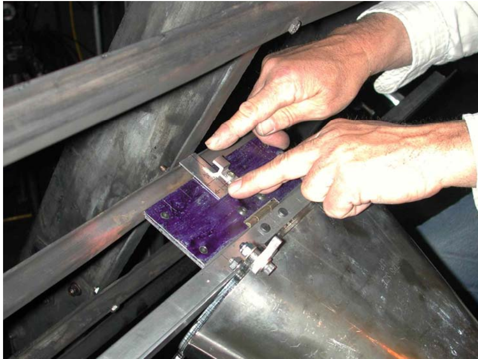
Figure 13. Aligning Burner with Center Former Using Drop-Down Tool
