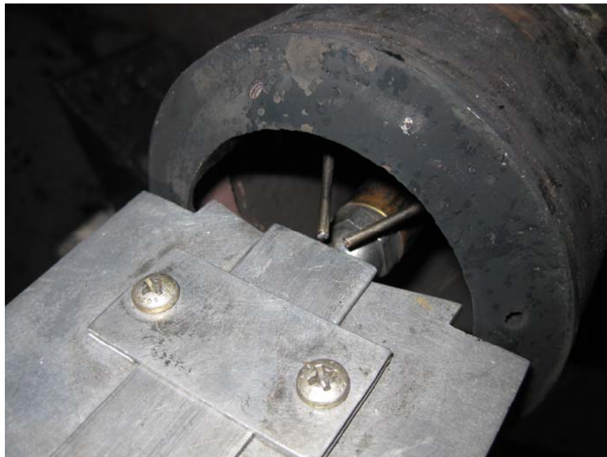
Figure 1. Depth Tool Seated Against Face of Turbulator (cone removed)
