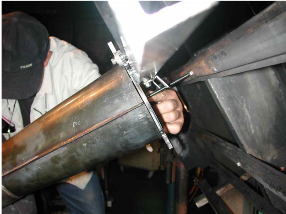
Figure 9. Setting Burner to Sample Holder Distance Using Bushing and Pointer
