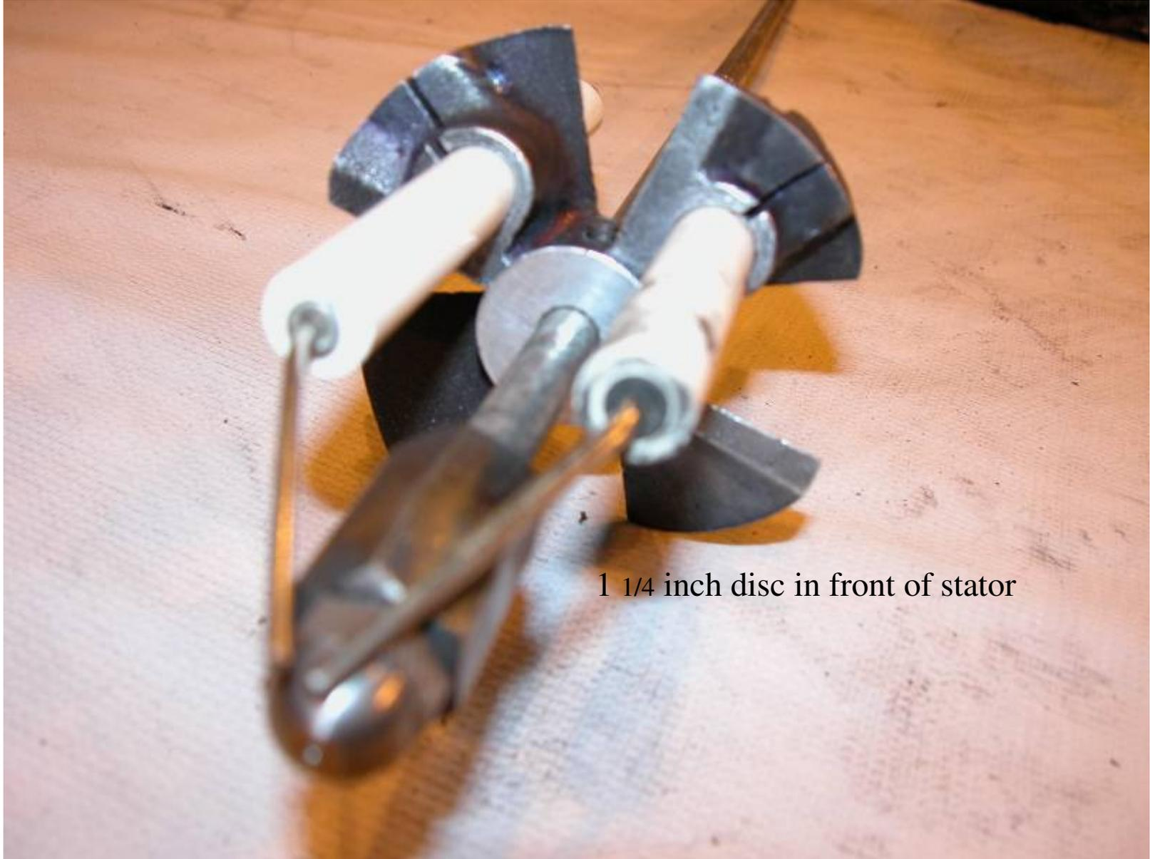
1 1/4 inch disc in front of stator
