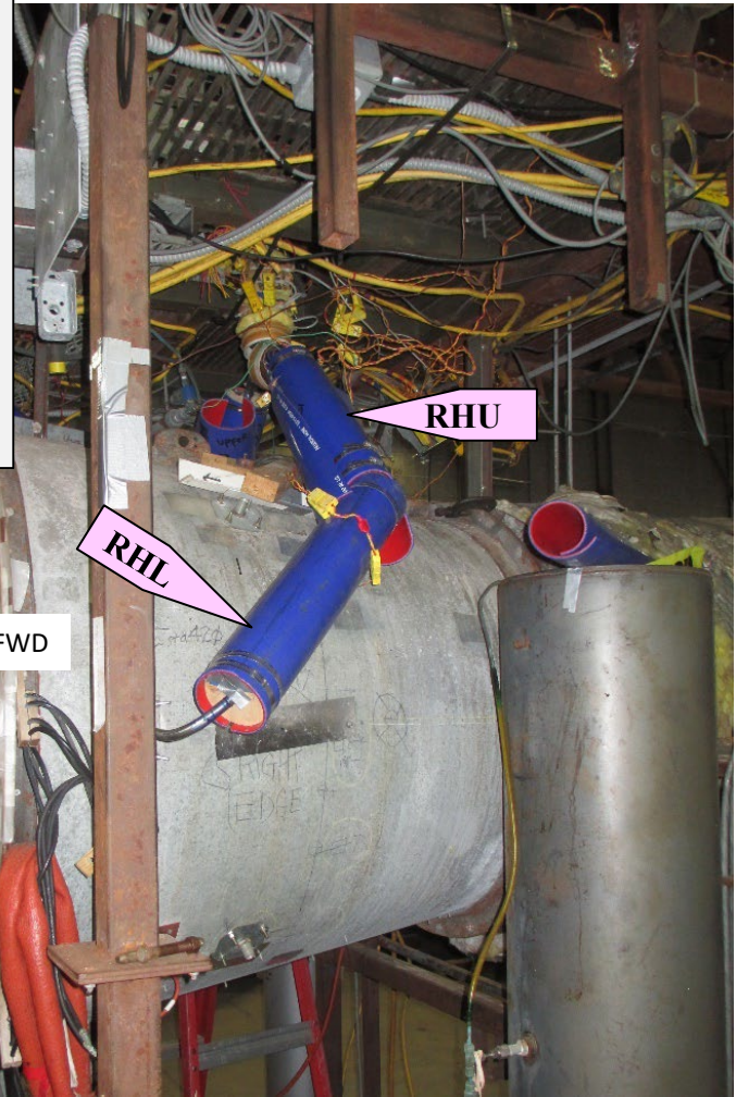
Left Firex Injection Branch Line, cold region [mid], surface thermocouple
