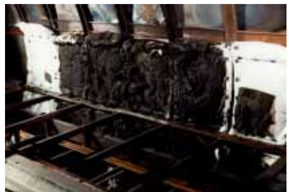
Burn Test with Effective Insulation
