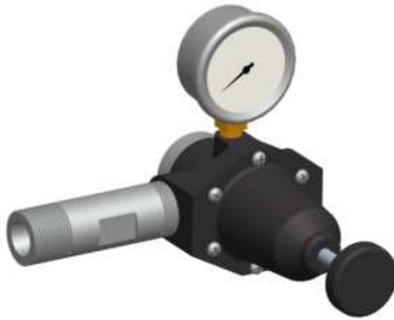
Figure 8-S-9. Schematic of Air Pressure Regulator with Sonic Nozzle Attached
