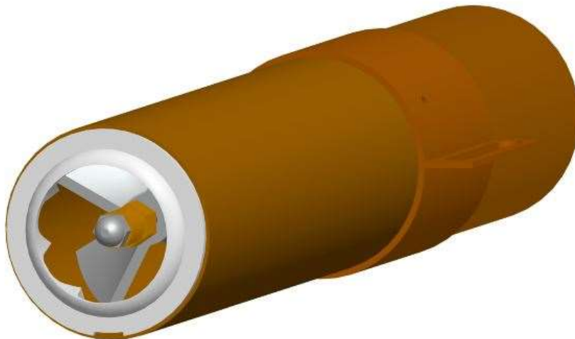
Figure 7-S-16. Position of Turbulator at the end of the Draft Tube
