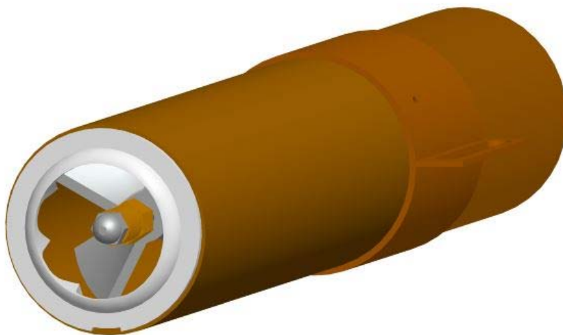
Figure 24-S-16. Position of Turbulator at the end of the Draft Tube
