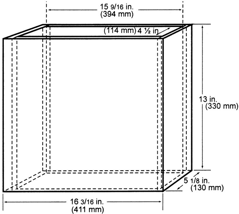
Figure 2 - Internal Chimney
