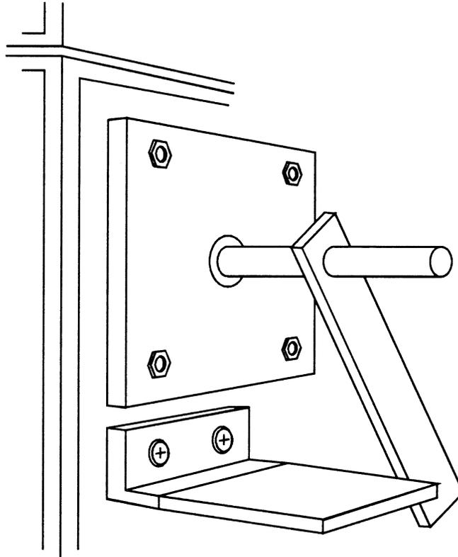
Figure 8 - Propane Burner Stop
