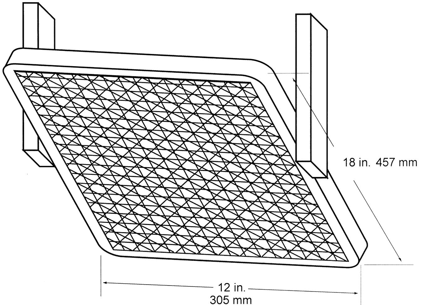
Figure 3b – Air Propane Radiant Panel
