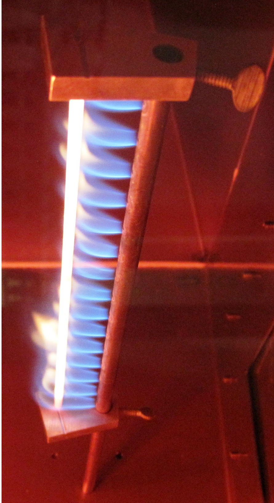
Figure 4. HSI / Upper Pilot Burner Operation
