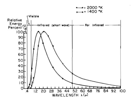
Figure 3. Spectral distribution of source energy.
