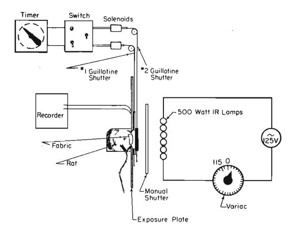
Figure 1. Thermal irradiation apparatus.
