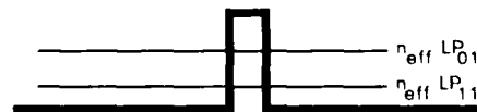
Fig. 1 Profile of a Matched Clad Fiber along with Effective Indices of Refraction of the LP 01 and LP 11 Modes ( \lambda < \lambda_c )
