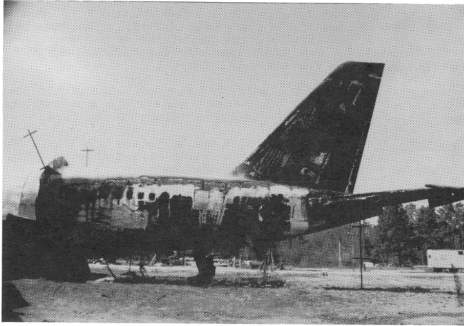
FIGURE 9. TEST 4 CV-880 PORT SIDE FIRE DAMAGE
