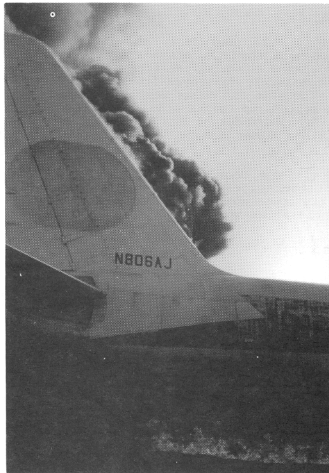
FIGURE 8. TEST 4 CV-800 STARBOARD SIDE FLAME EXPOSURE
