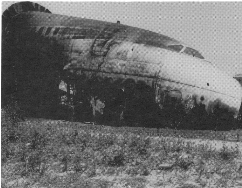
FIGURE 13. TEST 5 CV-880 STARBOARD SIDE FIRE DAMAGE
