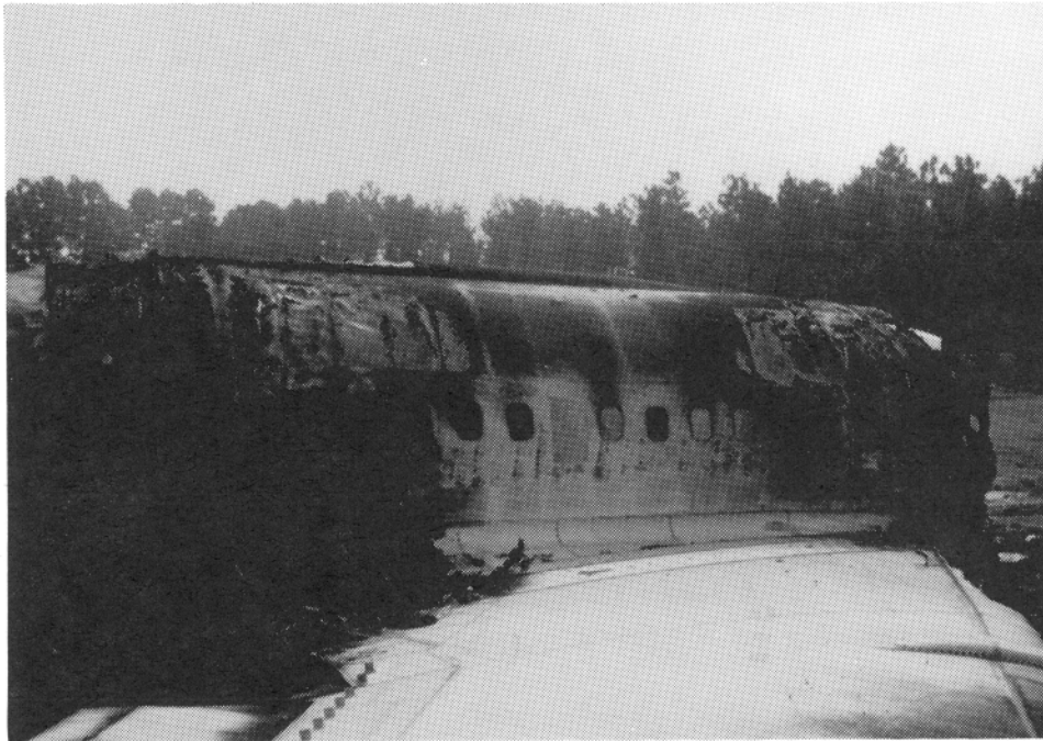
FIGURE 16. TEST 6 CV-880 STARBOARD SIDE FIRE DAMAGE
