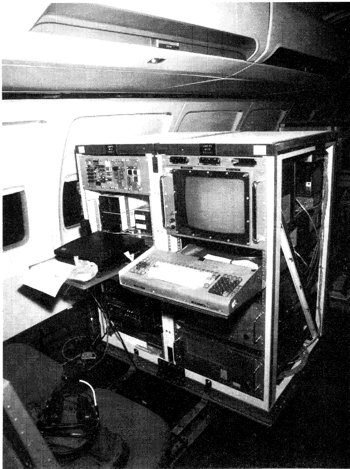
FIGURE 2.1.1-8 INSTRUMENT RACK, STATION 1548, LEFT SIDE
