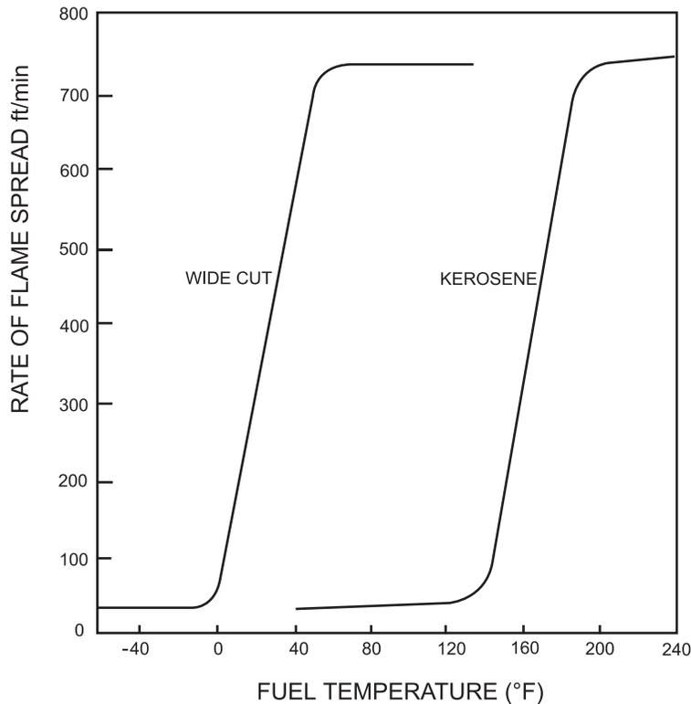
FIGURE 6. RATE OF SPREAD OF FLAME ACROSS A LAYER OF FUEL
