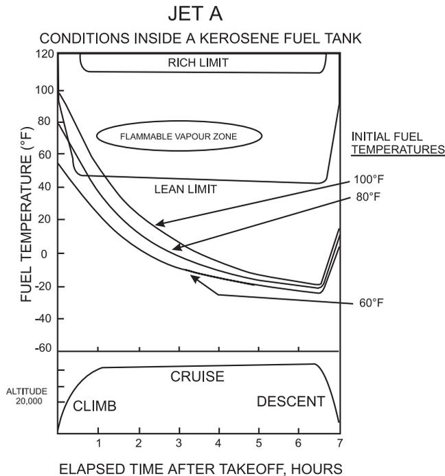
**FIGURE 7. TYPICAL JET A FUEL TEMPERATURES IN FLIGHT—JET TRANSPORT CRUISING AT 525 MPH. BASED ON BOEING AIRPLANE COMPANY AND DEHAVILLAND AIRCRAFT COMPANY, LTD. DATA**
