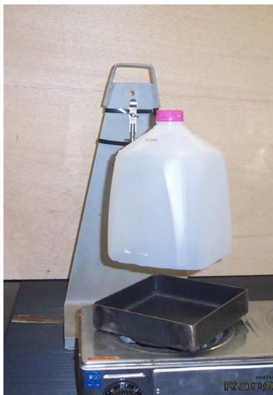
Figure 2. Vapor Ignition Test Setup
