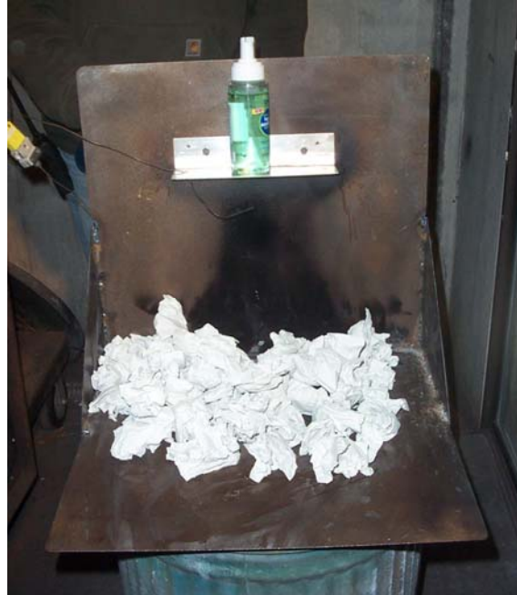
Figure 3. Paper Towel Burn Test Setup
