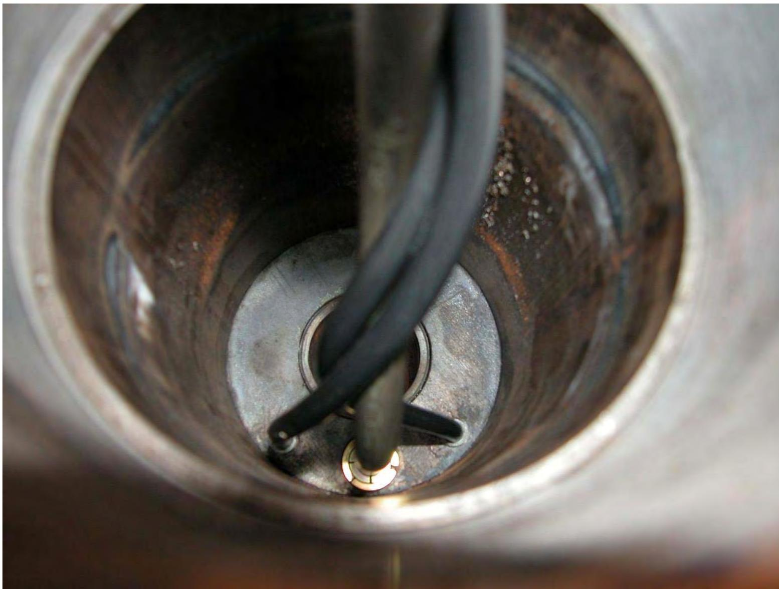
Figure A-9. Photograph of the Igniter Wires From Below
