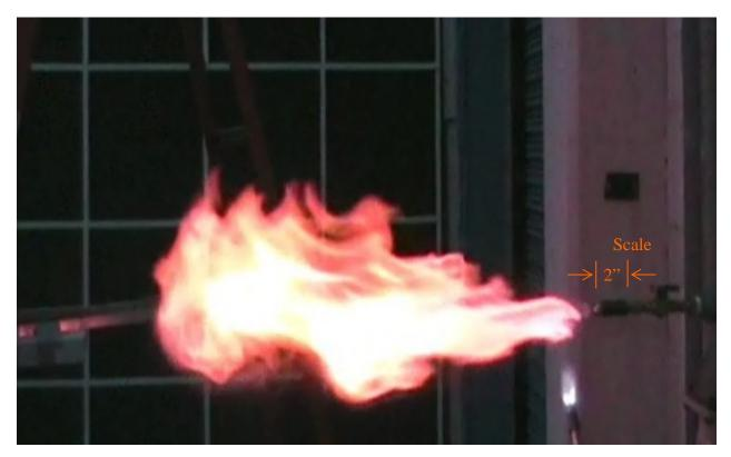
Figure 3. Observed Fire Plume From the Misting of TKS Anti-Icing Fluid in the Presence of an Ignition Source
