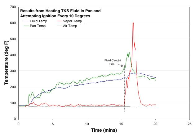
Figure 2. Measured Temperatures Obtained From Heating a Pan of TKS Anti-Icing Fluid and Applying an Ignition Source
