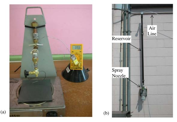
Figure 1. (a) Hot-Surface Flammability Test Apparatus and (b) Spray Flammability Test Apparatus
