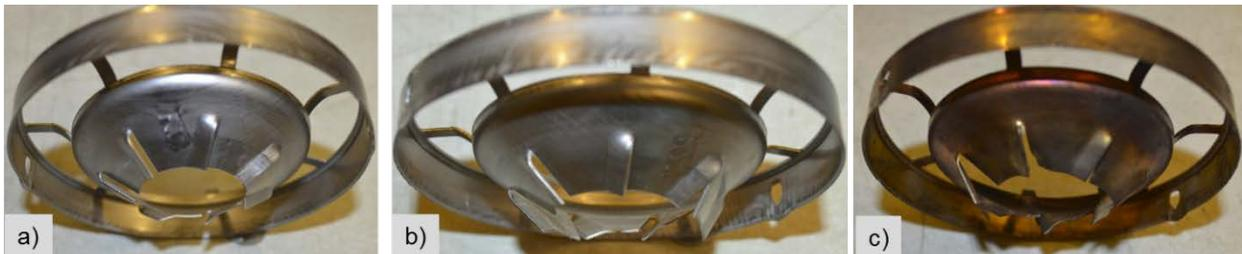
**Figure 62. Deformation of FRH: a) baseline (undamaged), b) slightly deformed, and c) severely deformed**
