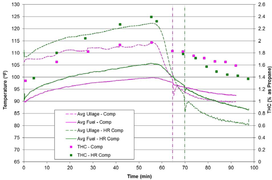
**Figure 13. Comparison of high-reflectivity and bare composite material fuel tank results for a 40% fuel load under the low-heat setting**
