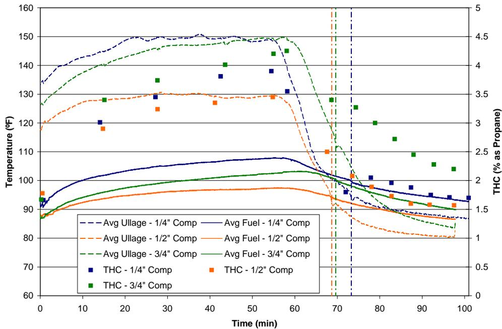
**Figure 20. Comparison of various thickness composite material fuel tank results for an 80% fuel load under the high-heat setting**
