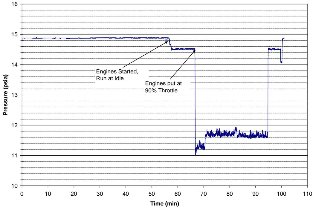
**Figure 1. Typical pressure profile of fuel tank during wind tunnel operations**
