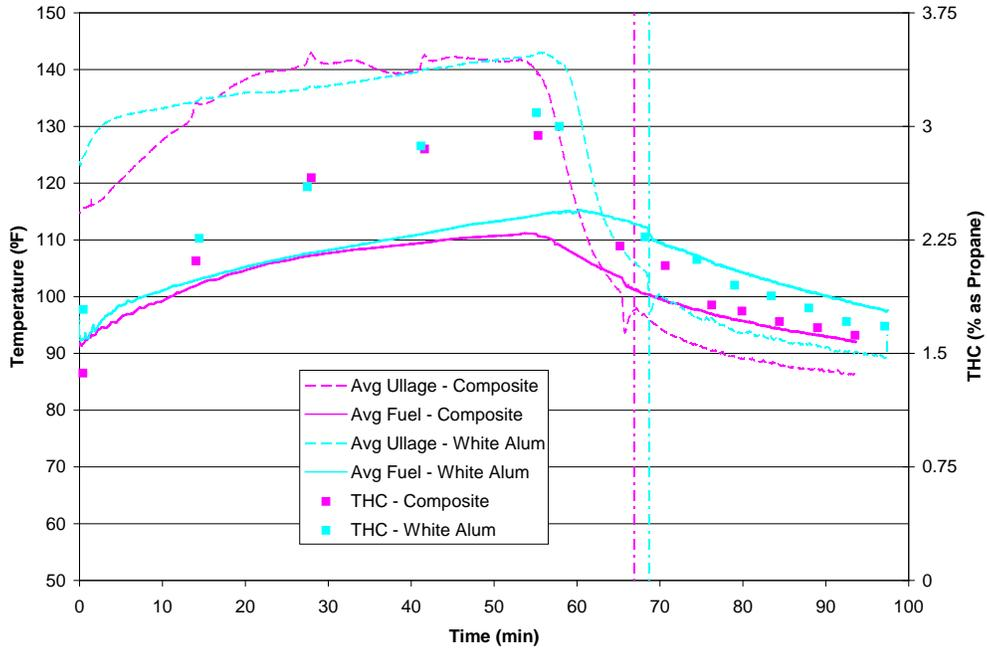
**Figure 9. Comparison of white-painted aluminum and bare composite material fuel tank results for a 40% fuel load under the high-heat setting**
