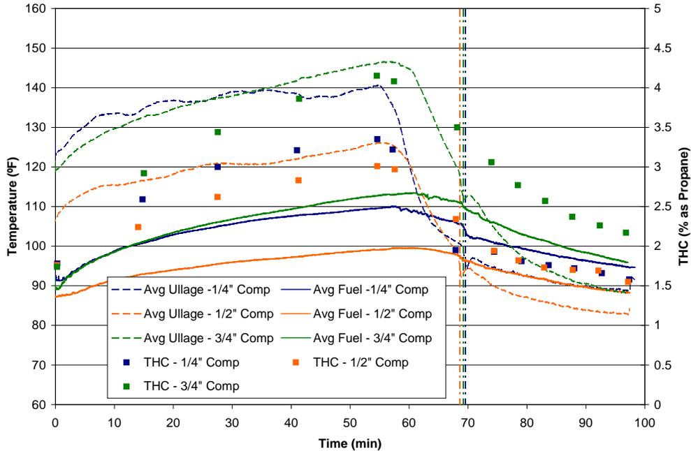
**Figure 19. Comparison of various thickness composite material fuel tank results for a 40% fuel load under the high-heat setting**
