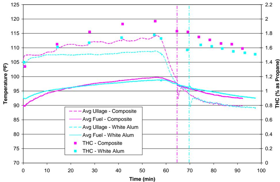
**Figure 6. Comparison of white-painted aluminum and bare composite material fuel tank results for a 40% fuel load under the low-heat setting**
