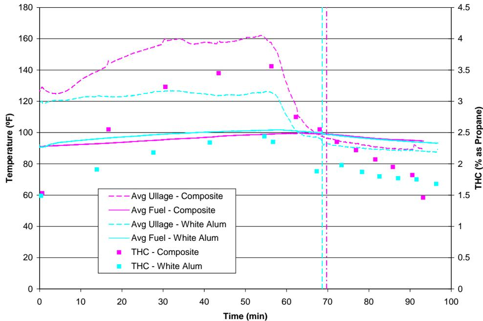
**Figure 11. Comparison of white-painted aluminum and bare composite material fuel tank results for an 80% fuel load under the high-heat setting**
