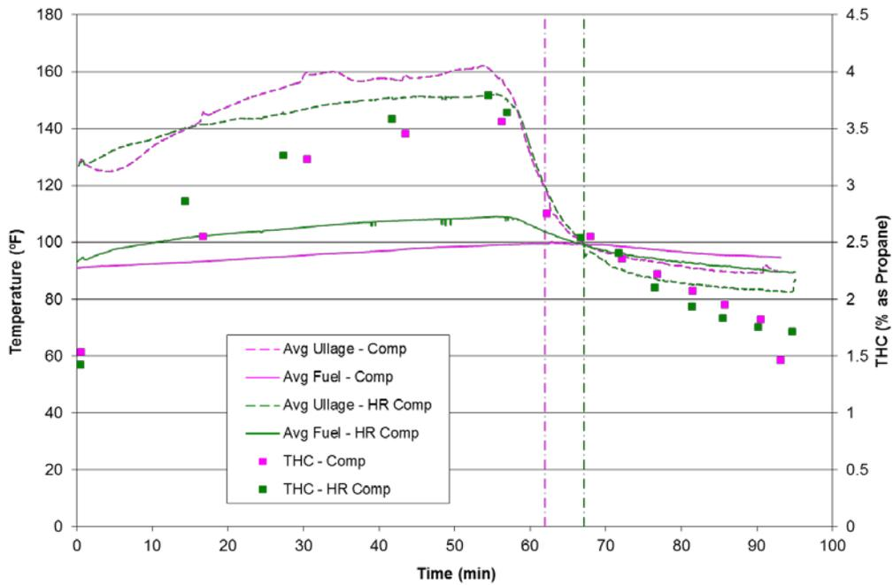
**Figure 16. Comparison of high-reflectivity and bare composite material fuel tank results for an 80% fuel load under the high-heat setting**
