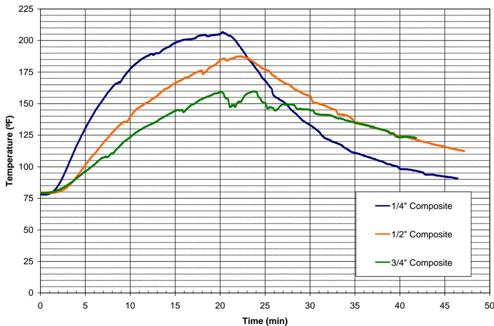
**Figure 5. Comparison of center-point temperature for the various thickness composite materials during panel heating test**
