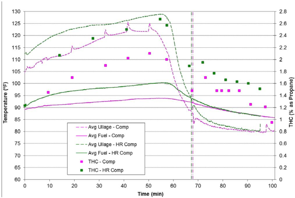
**Figure 15. Comparison of high-reflectivity and bare composite material fuel tank results for an 80% fuel load under the low-heat setting**
