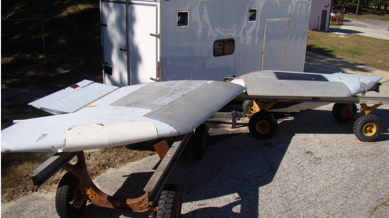
**Figure 2. 727 wing tank test articles**
