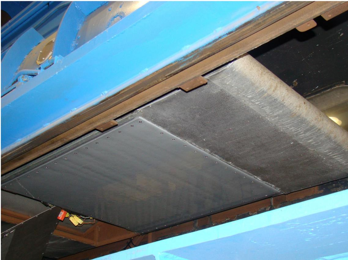
**Figure 12. Photograph of tank with high-reflectivity aluminum epoxy applied to composite material**
