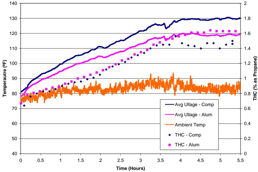
**Figure 21. 727 wing tank test results for a 5.5-hour test started in early morning**
