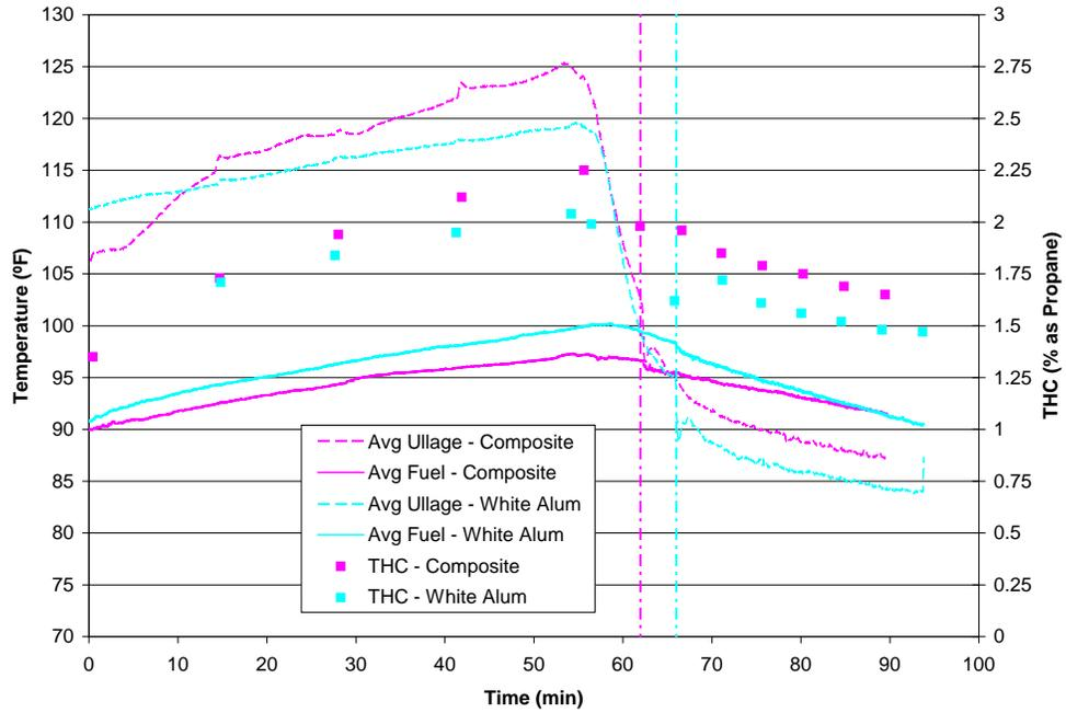
**Figure 7. Comparison of white-painted aluminum and bare composite material fuel tank results for a 60% fuel load under the low-heat setting**
