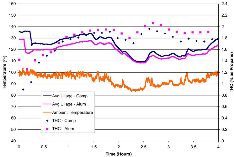
**Figure 22. 727 wing tank test results for a 4-hour test started mid-morning**
