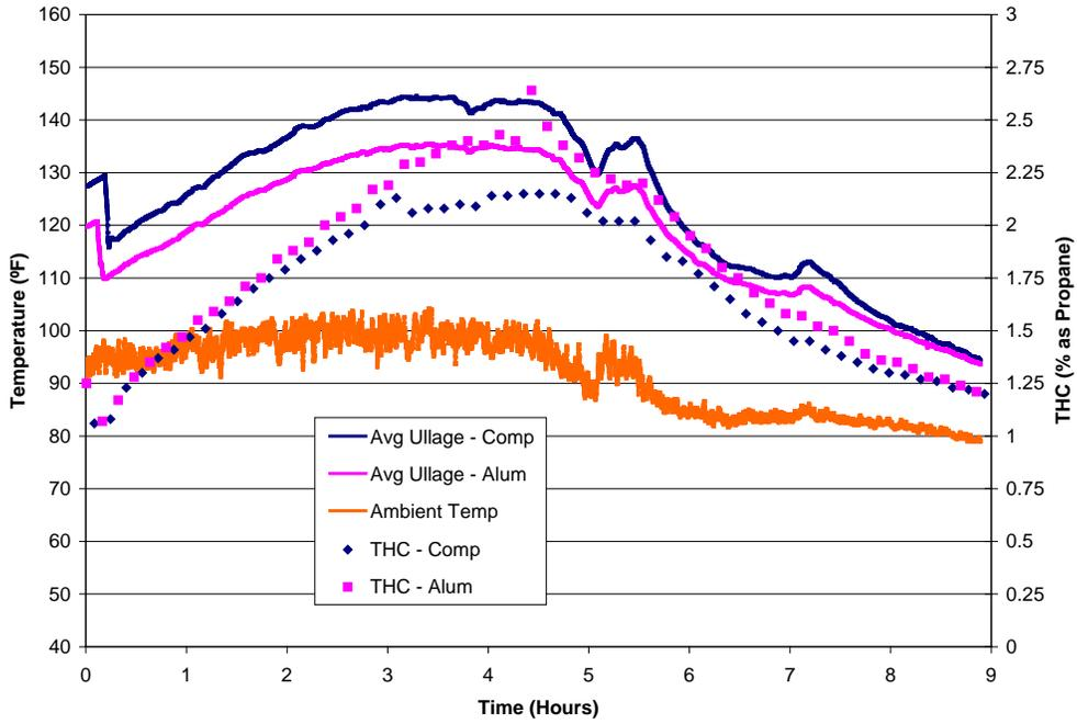
**Figure 23. 727 wing tank test results for a 9-hour test started mid-morning**
