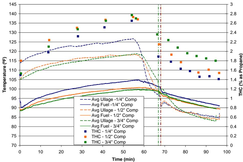
**Figure 17. Comparison of various thickness composite material fuel tank results for a 40% fuel load under the low-heat setting**
