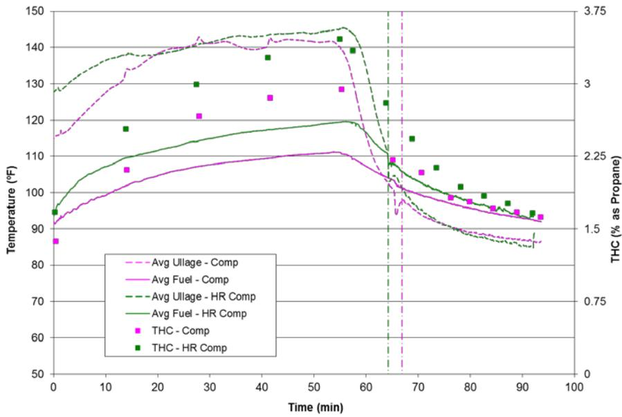
**Figure 14. Comparison of high-reflectivity and bare composite material fuel tank results for a 40% fuel load under the high-heat setting**
