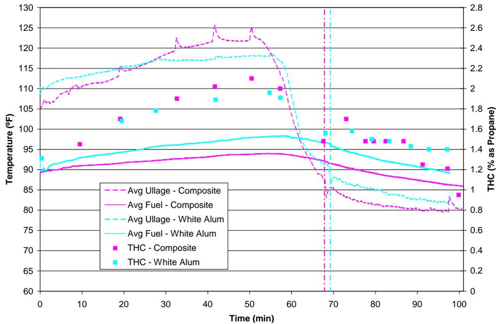
**Figure 8. Comparison of white-painted aluminum and bare composite material fuel tank results for an 80% fuel load under the low-heat setting**
