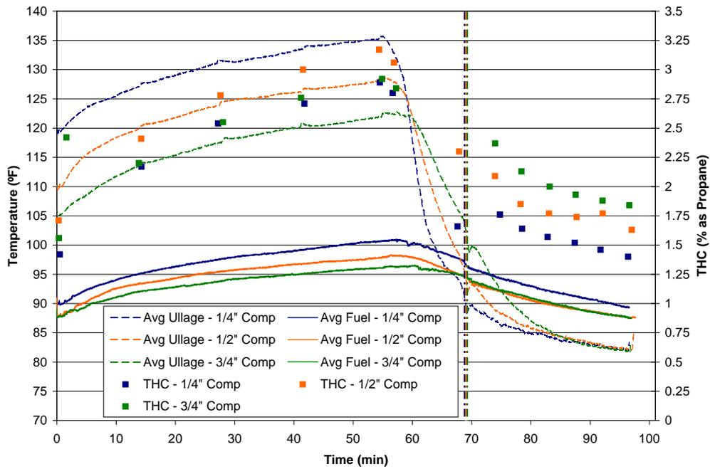
**Figure 18. Comparison of various thickness composite material fuel tank results for an 80% fuel load under the low-heat setting**
