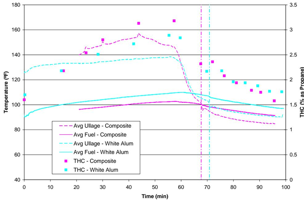
**Figure 10. Comparison of white-painted aluminum and bare composite material fuel tank results for a 60% fuel load under the high-heat setting**
