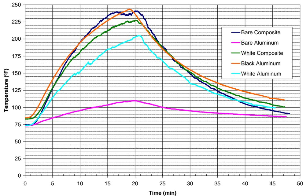
**Figure 4. Comparison of center-point temperature for the bare and painted composite and aluminum materials during panel-heating test**
