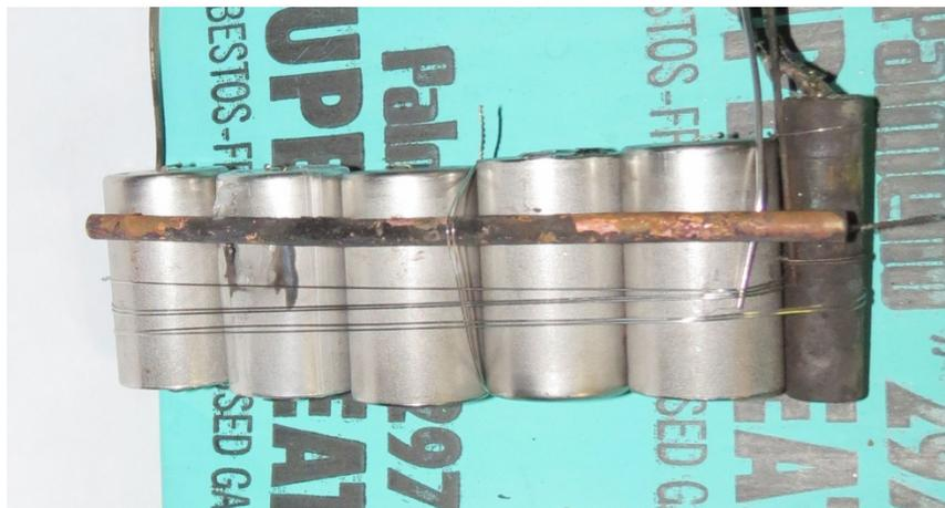
**Figure 8. Cylindrical-cell propagation test setup**
