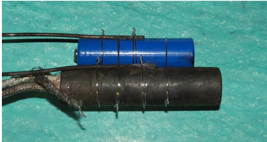
**Figure 6. Single-cell thermal runaway setup for cylindrical cell types**
