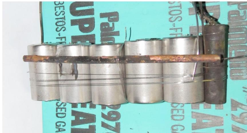
**Figure 8. Cylindrical-cell propagation test setup**
