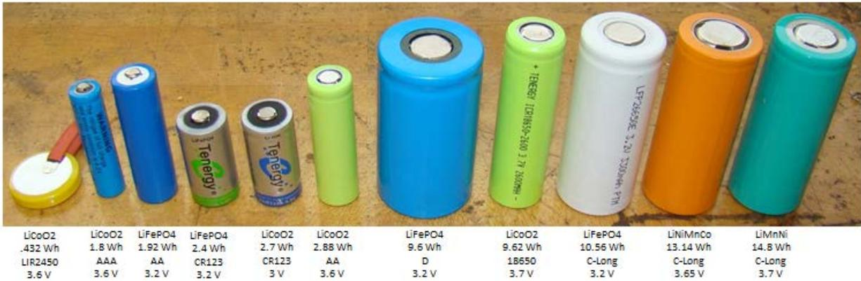
Figure 3. Photograph showing the lithium-ion cells that were tested
