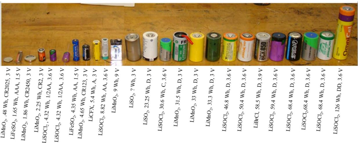
Figure 5. Photograph showing the lithium-metal cells that were tested
