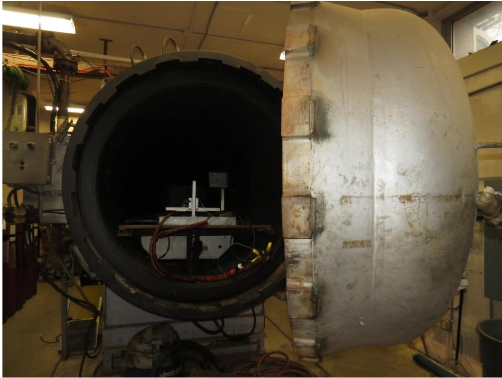
**Figure 1.** The  $10.8 \text{ m}^3$  pressure vessel
