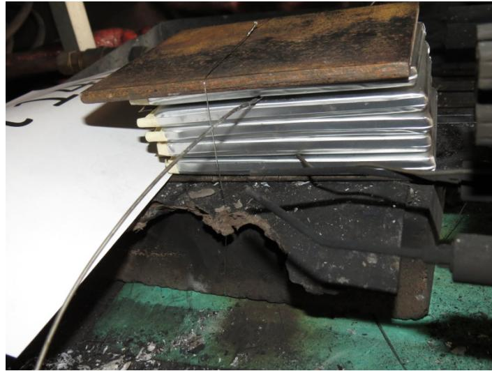
**Figure 9. Pouch-cell propagation test setup**
