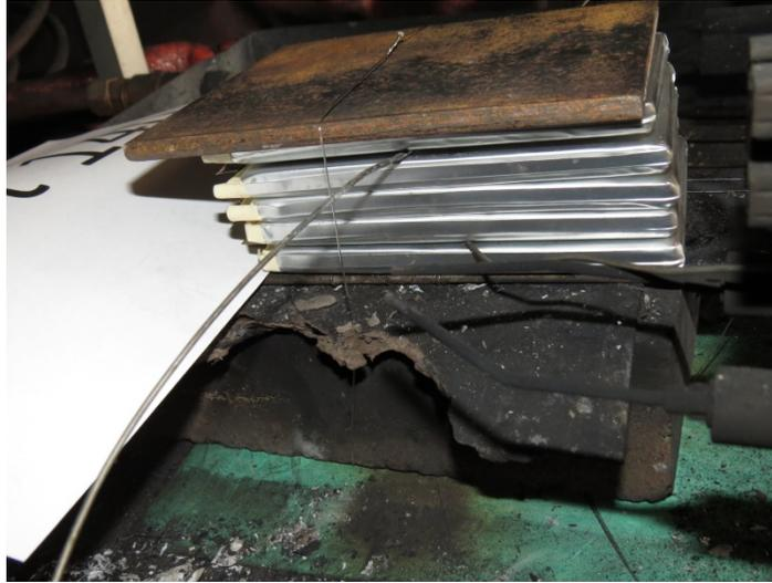
**Figure 9. Pouch-cell propagation test setup**
