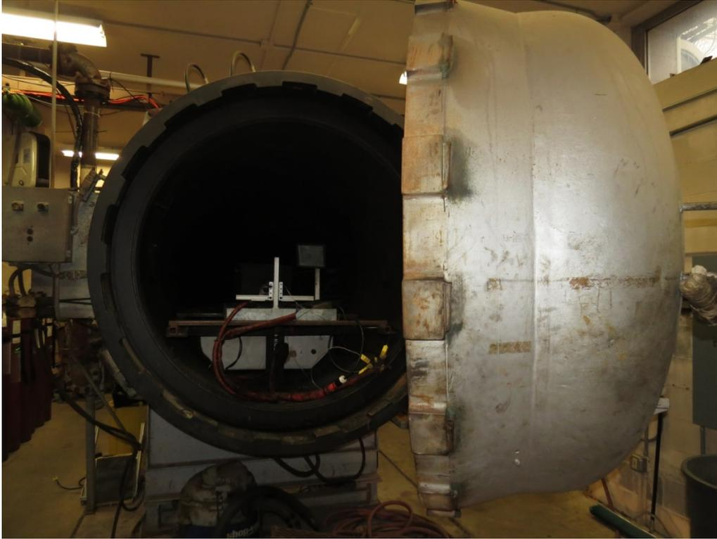
**Figure 1. The 10.8 m<sup>3</sup> pressure vessel**
