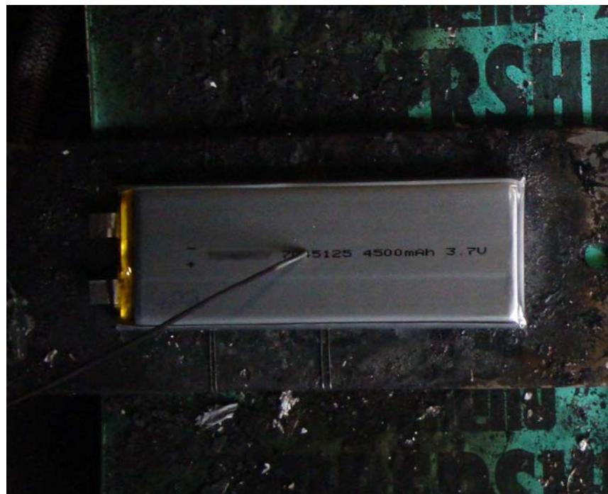
**Figure 7. Single-cell thermal runaway setup for pouch cell types**
