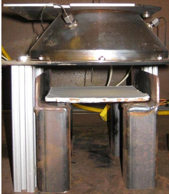
**Figure 12. Setup of a radiant heat source test**
