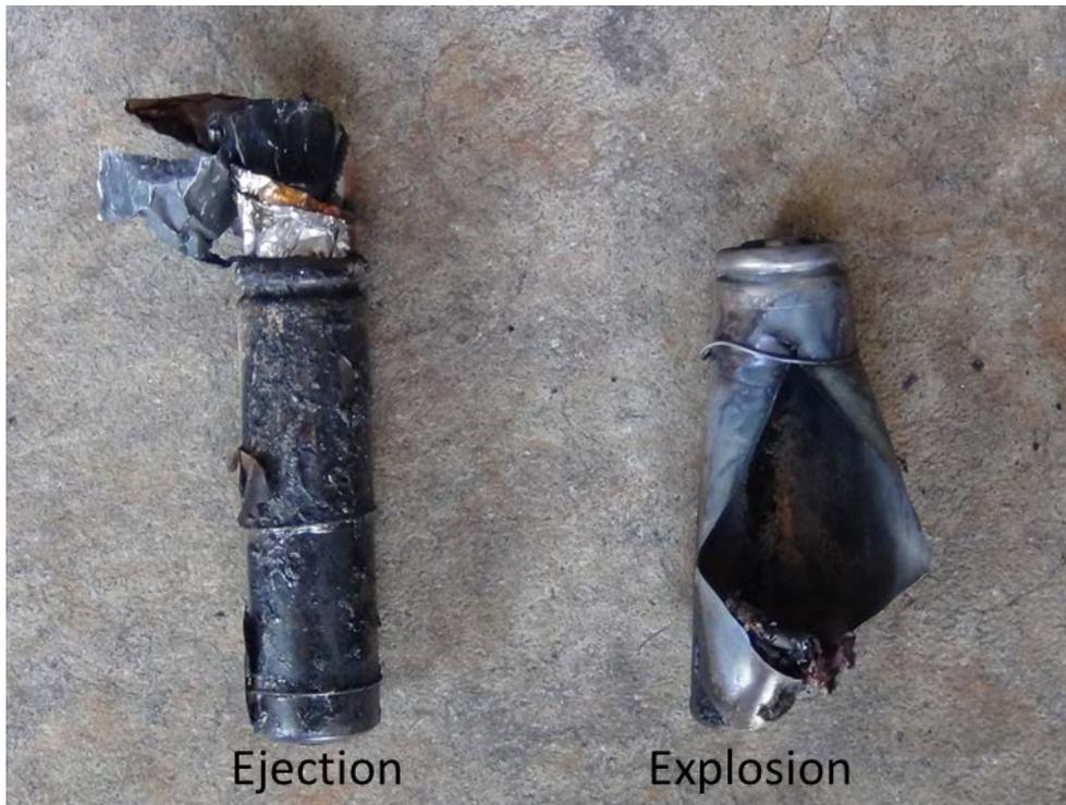
**Figure 27. 18650 cell with ejected inner materials**
