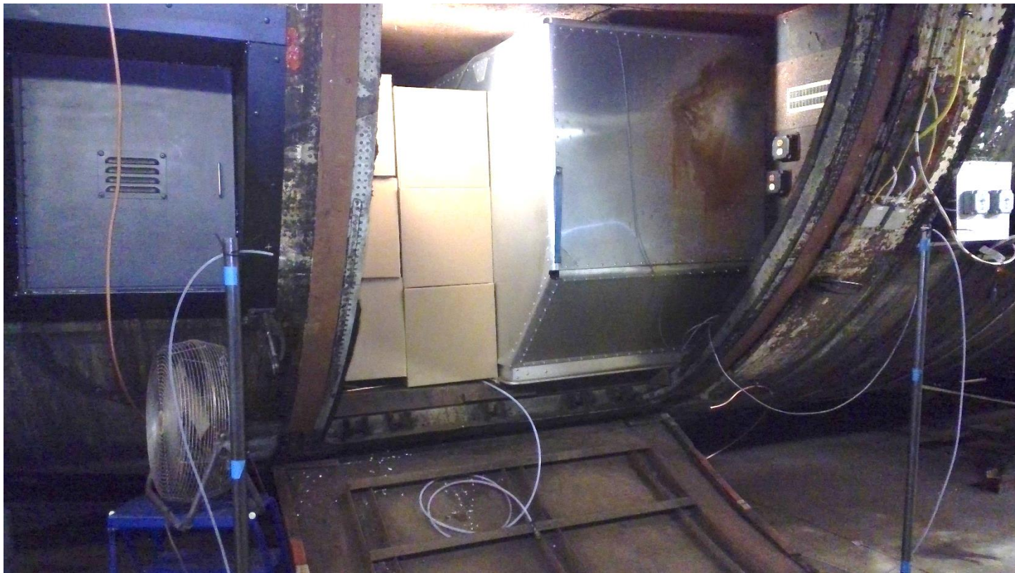
Test Compartment Loaded with LD3 Containers and Fan Located AFT of the Cargo Door
