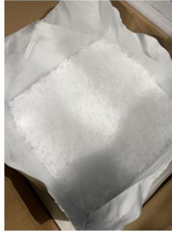
Dry ice pellets held in bag above the internal payload area.
