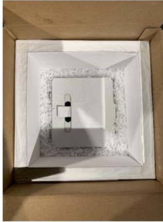
Dry ice pellets filled around the internal payload area.
