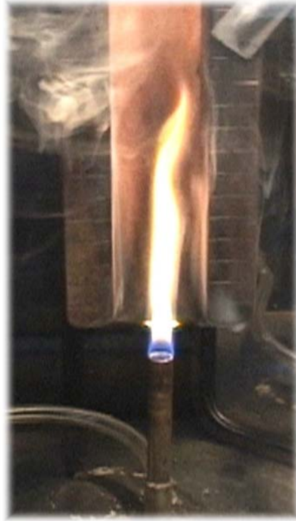
Figure 1b. Vertical Bunsen Burner Test Method
