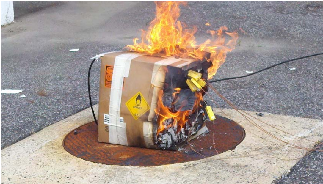
Chemical Oxygen Generator Overpack tested with 100 lithium metal cells.
