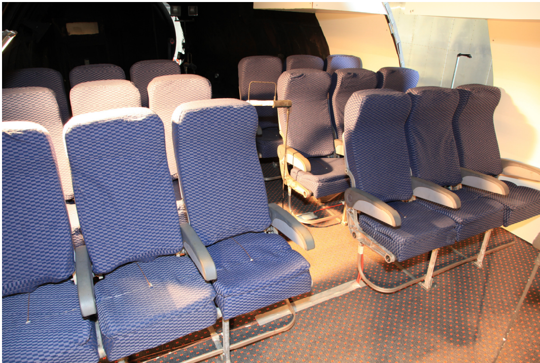
Interior of Test Fuselage Showing three Rows of Magnesium-Framed Aircraft Seats
