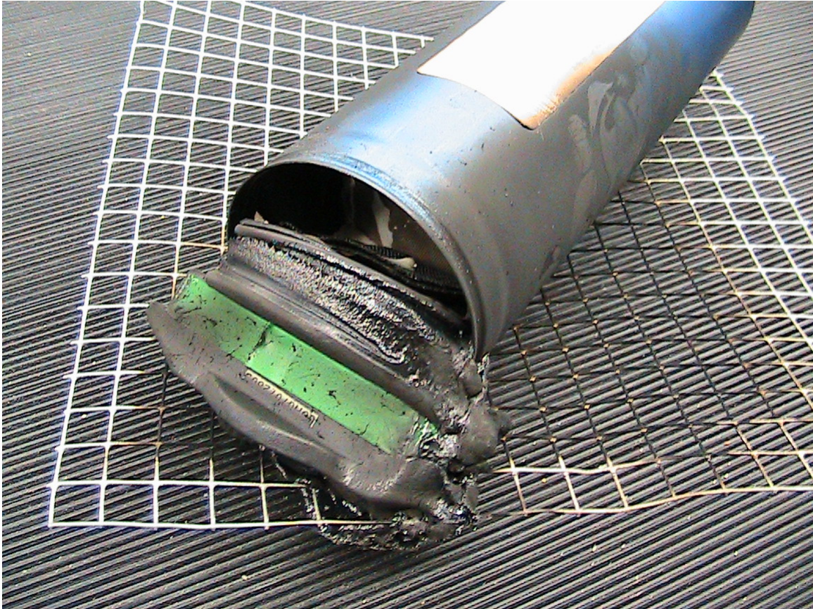
Post Fire Test Photograph of Sodium Borohydride Fuel Cell Cartridge
