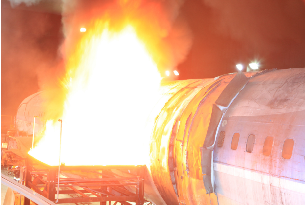
Full-Scale Fire Test on Magnesium-Framed Aircraft Seats
