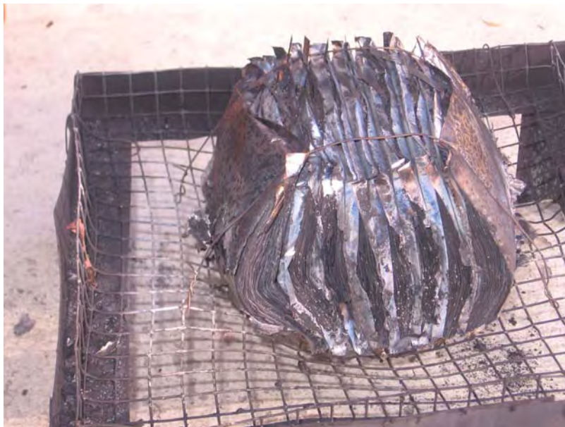
Figure 13. Results From the Eight-Cell Test of Battery Type 3
