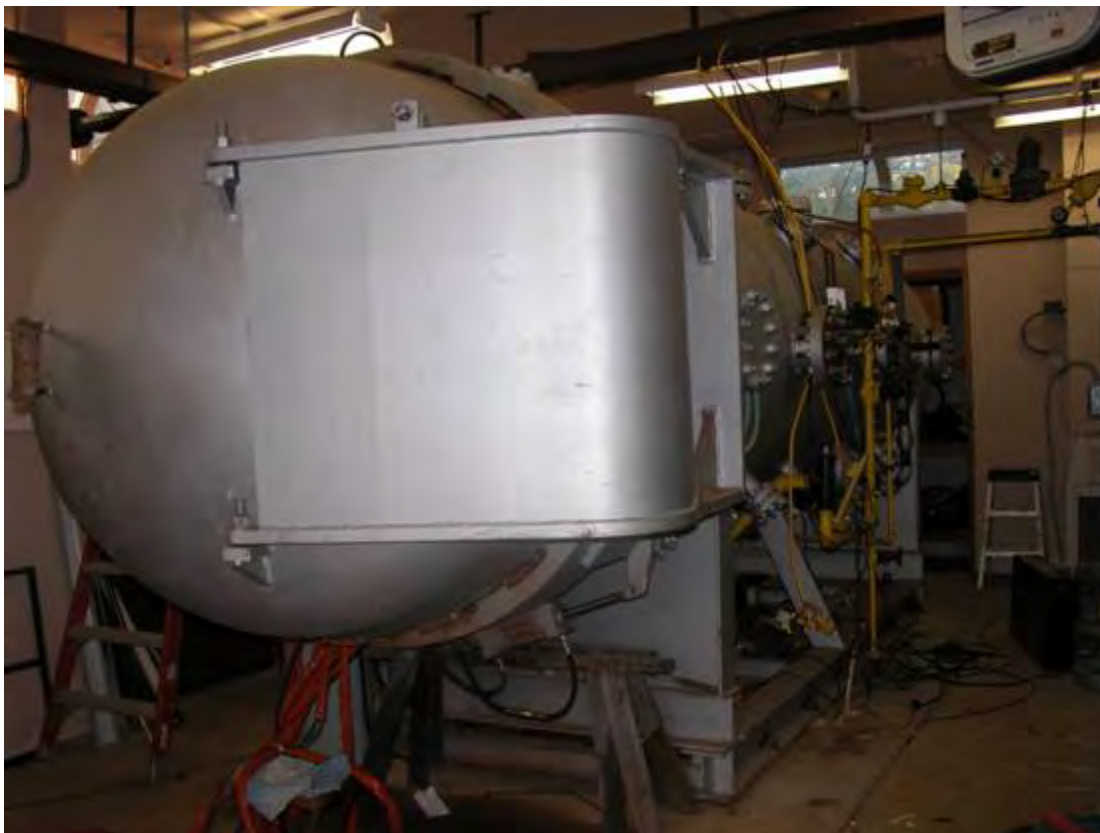
Figure 4. External View of the Pressure Fire Modeling Facility
