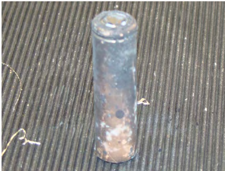
Figure 8. Results From the Single-Cell Test of Battery Type 1
