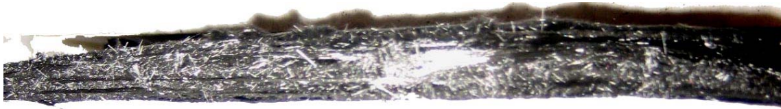
Figure 23. Cross Section of the 40 kW/m 2 Heated Composite
