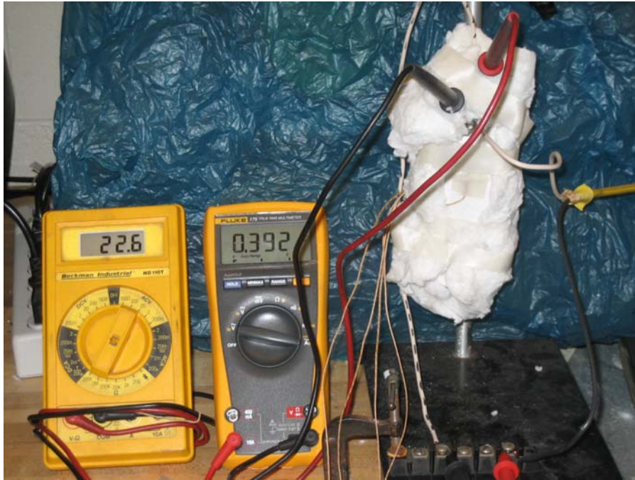
Figure 2. Conduction Apparatus: Heater Plate in Specimen Sandwich With Edge Insulation
