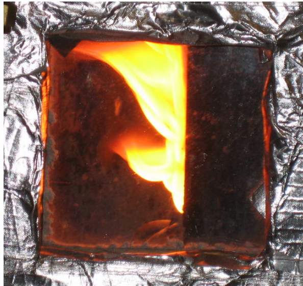
Figure 19. Vertical Burning in the OSU Apparatus
