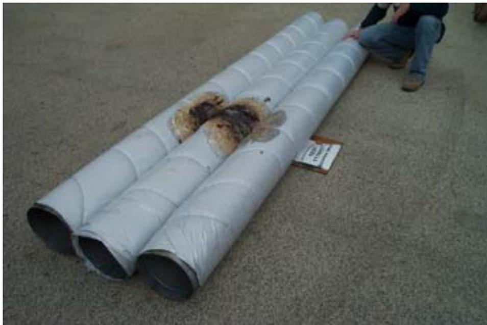
FIGURE 26. MPV TEST 6—POSTTEST PHOTOGRAPH OF DUCTS
