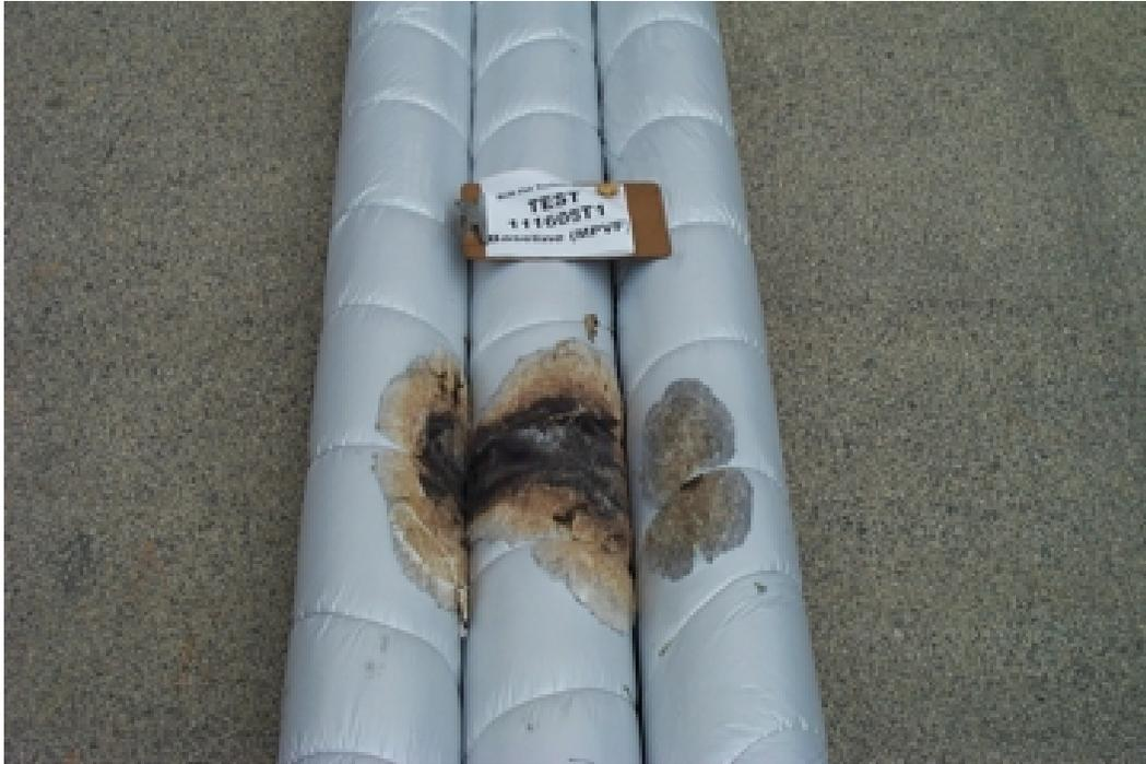
FIGURE 33. TEST 8—POSTTEST PHOTOGRAPH OF DUCTS
