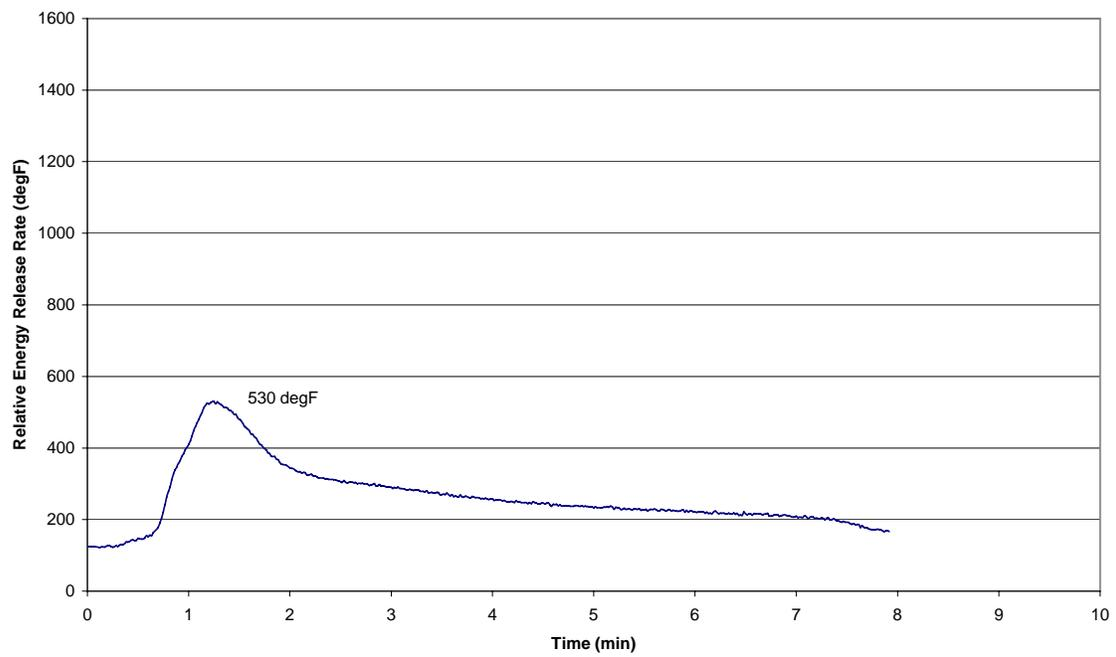
FIGURE 13. TEST 3—RELATIVE ENERGY RELEASE RATE VS TIME
