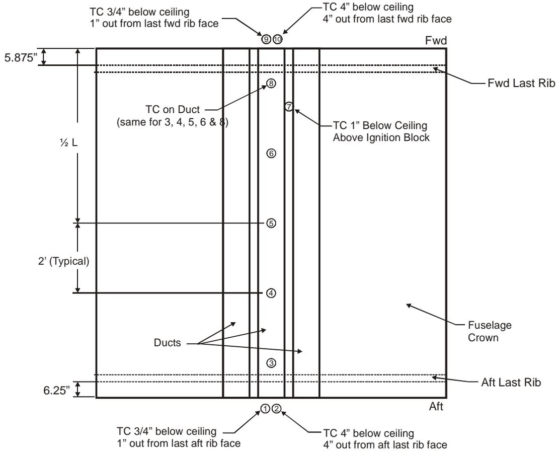
FIGURE 2. THERMOCOUPLE LOCATIONS
