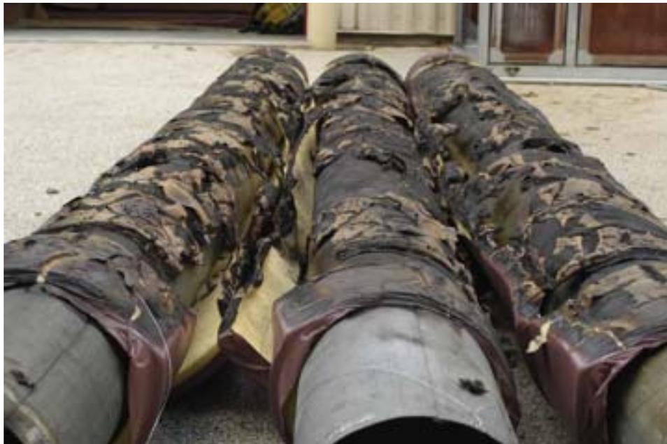
FIGURE 14. TEST 3—POSTTEST PHOTOGRAPH OF DUCTS
