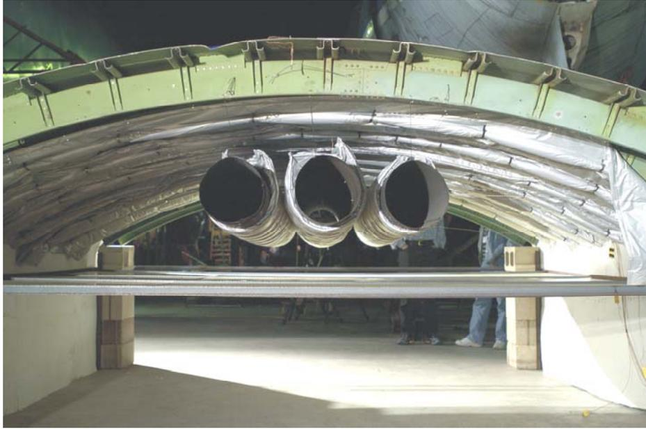
FIGURE 1. FUSELAGE SECTION WITH DUCTS INSTALLED
