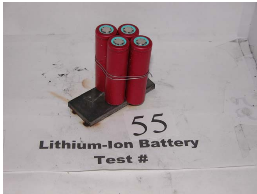
FIGURE 1. 18650 LITHIUM-ION CELLS PREPARED FOR TEST
