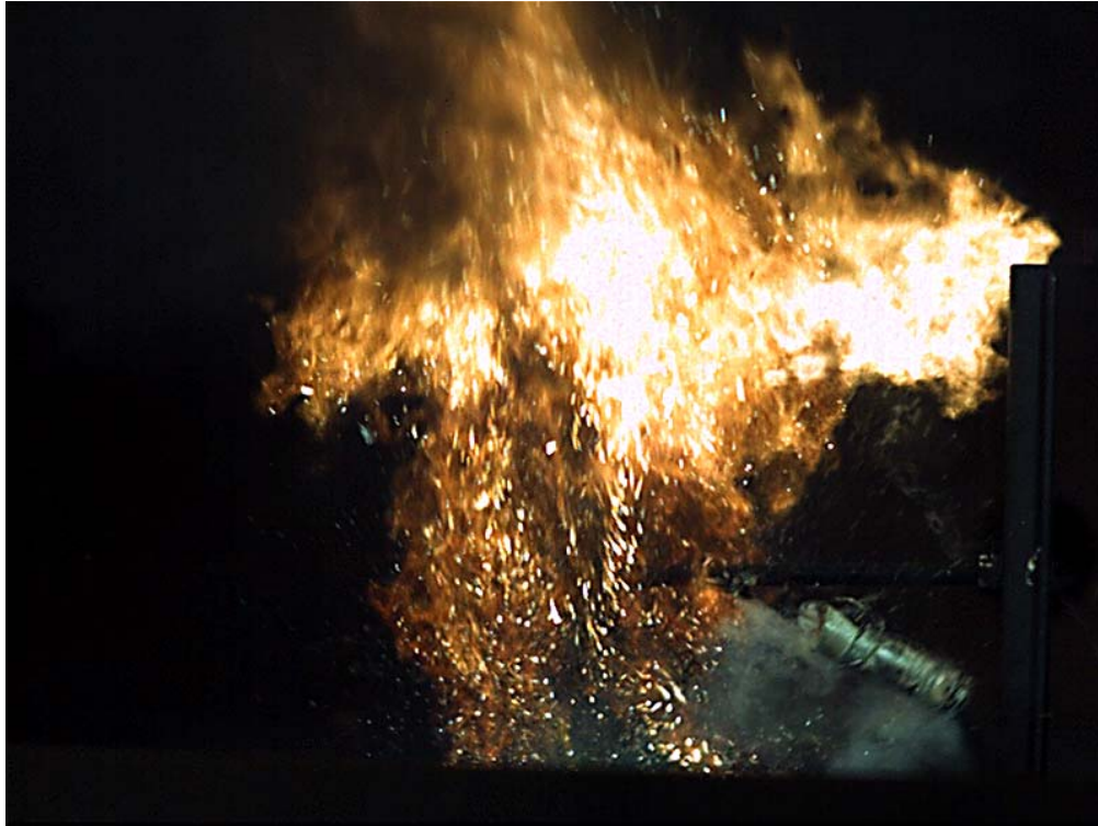
FIGURE 9. HIGH-SPEED VIDEO CAPTURE OF EXPLODING CELL
