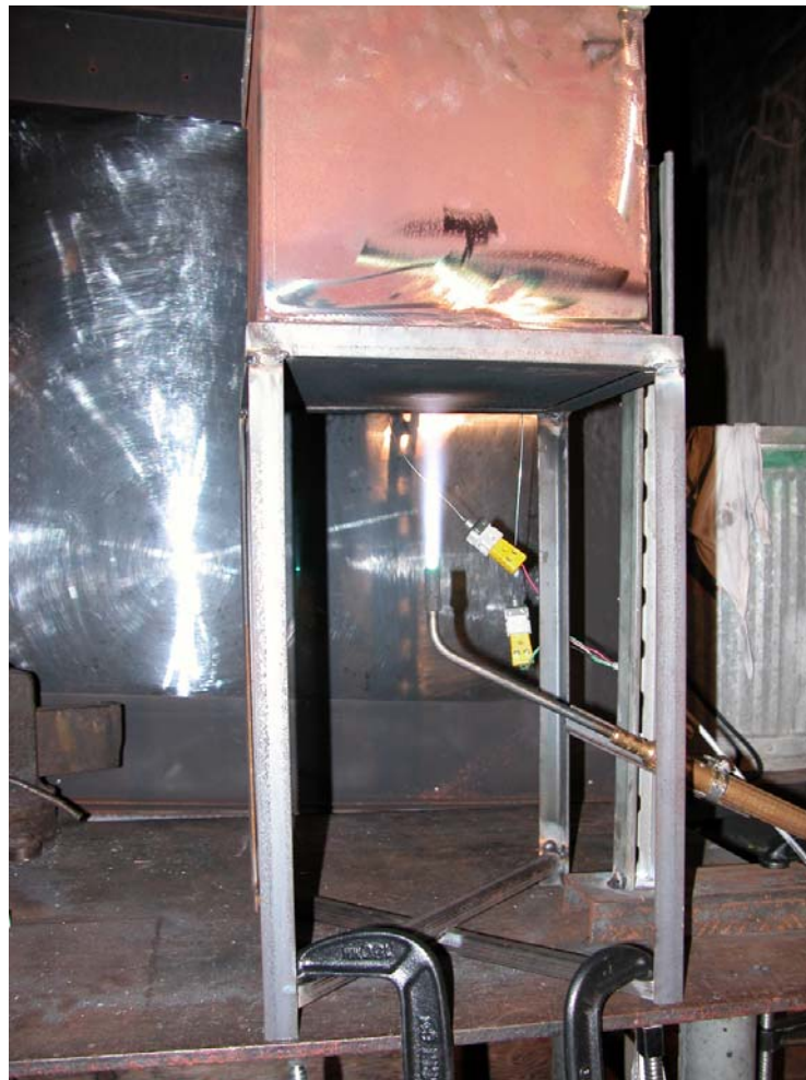
FIGURE 19. AUTOIGNITION TEST CHAMBER
