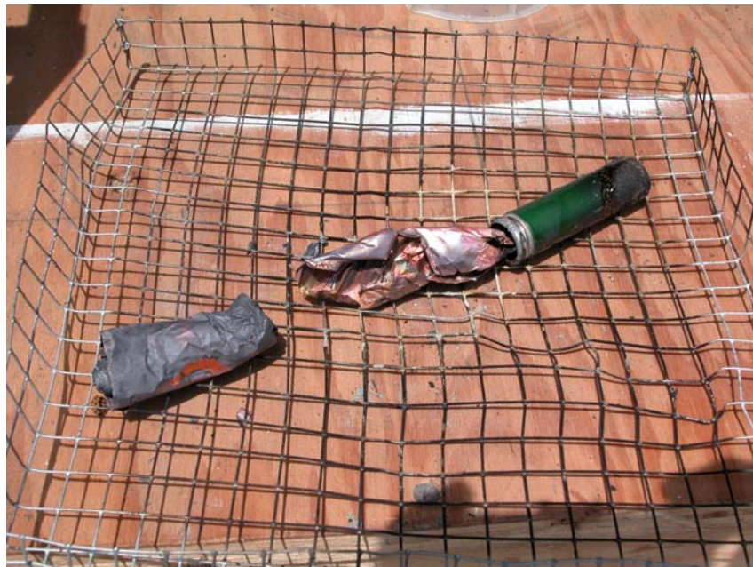
FIGURE 5. EXPLODED CELL AND ITS CONTENTS
