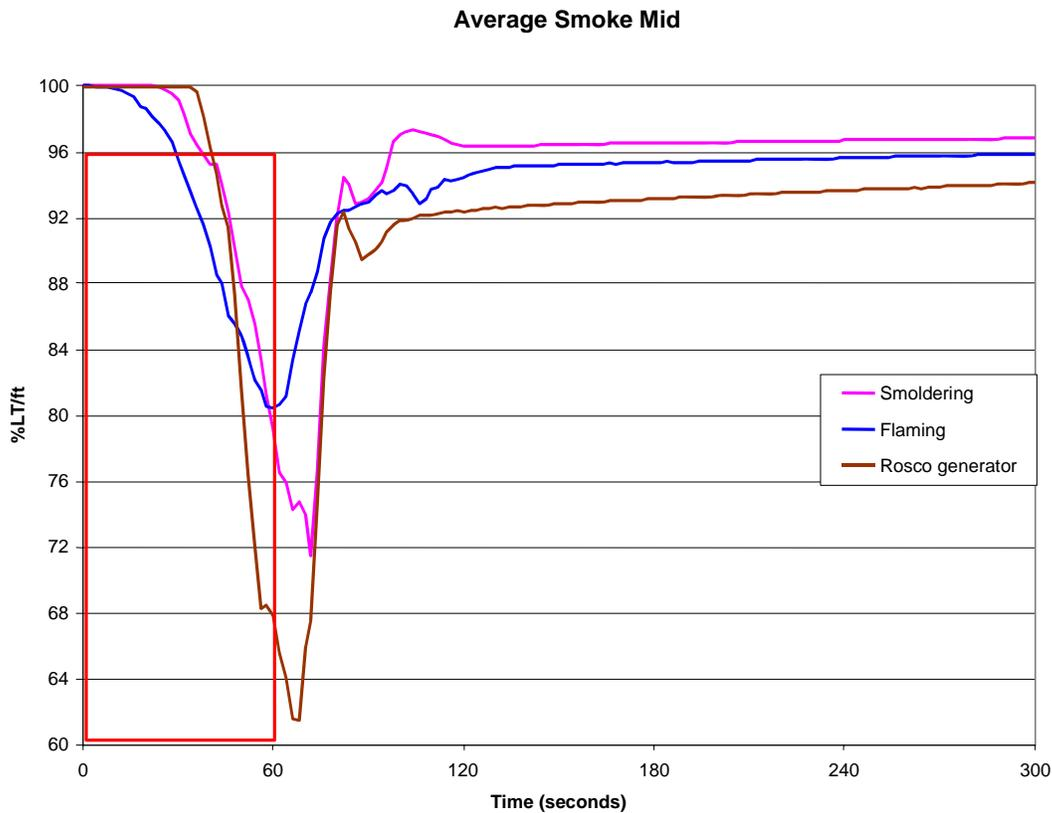
FIGURE 3. SMOKE OUTPUT FROM THREE FIRE SOURCES
