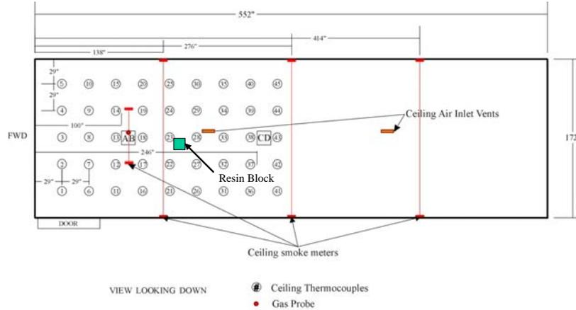
FIGURE 13. FLAMING RESIN NEAR THE CENTER OF DC-10 CARGO COMPARTMENT
