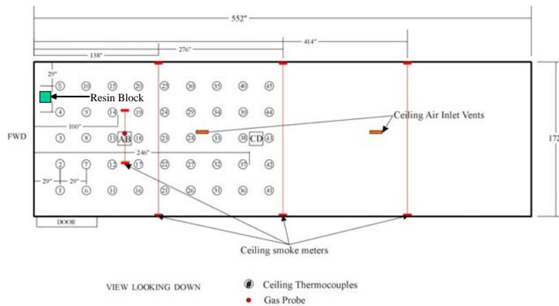
FIGURE 14. FLAMING RESIN IN THE FORWARD CORNER OF DC-10 CARGO COMPARTMENT
