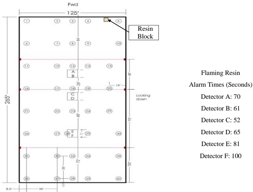
**FIGURE 7. FLAMING RESIN BLOCK IN THE FORWARD CORNER OF B-707 CARGO COMPARTMENT**
