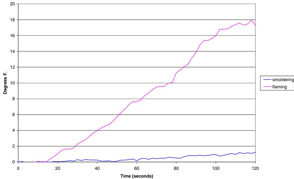
FIGURE 11. SMOLDERING AND FLAMING RESIN BLOCK CEILING TEMPERATURE RISE NEAR THE CENTER OF COMPARTMENT
