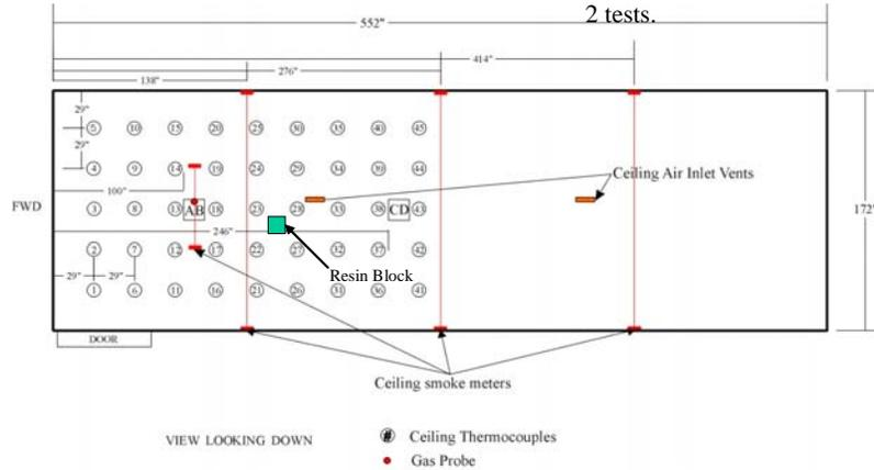
FIGURE 15. SMOLDERING RESIN NEAR THE CENTER OF DC-10 CARGO COMPARTMENT
