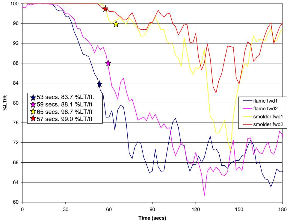
FIGURE 23. SMOKE LEVELS AT DETECTOR ALARM TIME FOR FLAMING AND SMOLDERING FIRES IN THE FORWARD CORNER OF THE DC-10 COMPARTMENT
