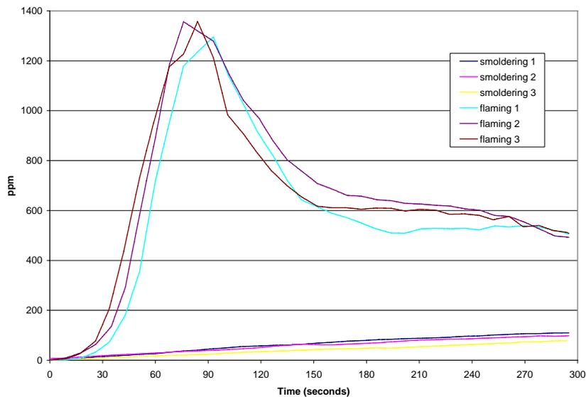
FIGURE 8. CARBON MONOXIDE FROM SMOLDERING AND FLAMING RESIN BLOCK
