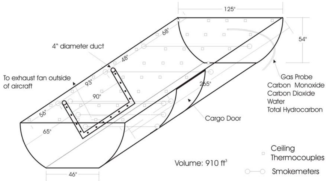
FIGURE 2. B-707 CARGO COMPARTMENT INSTRUMENTATION
