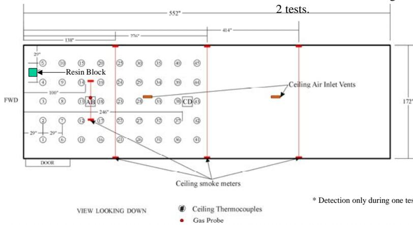
FIGURE 16. SMOLDERING RESIN IN THE FORWARD CORNER OF DC-10 CARGO COMPARTMENT
