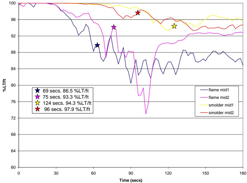
FIGURE 22. SMOKE LEVELS AT DETECTOR ALARM TIME FOR FLAMING AND SMOLDERING FIRES NEAR THE MIDDLE OF THE DC-10 COMPARTMENT
