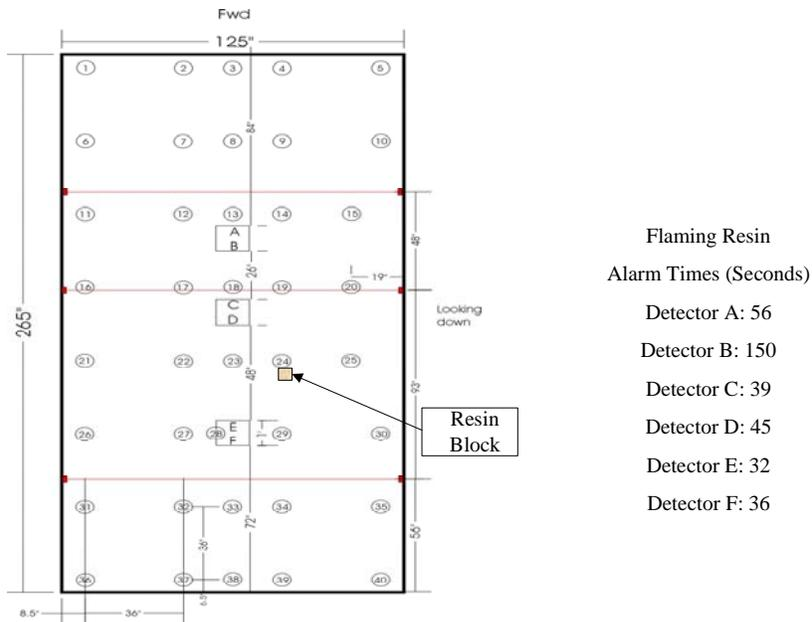
**FIGURE 6. FLAMING RESIN BLOCK NEAR THE CENTER OF B-707 CARGO COMPARTMENT**
