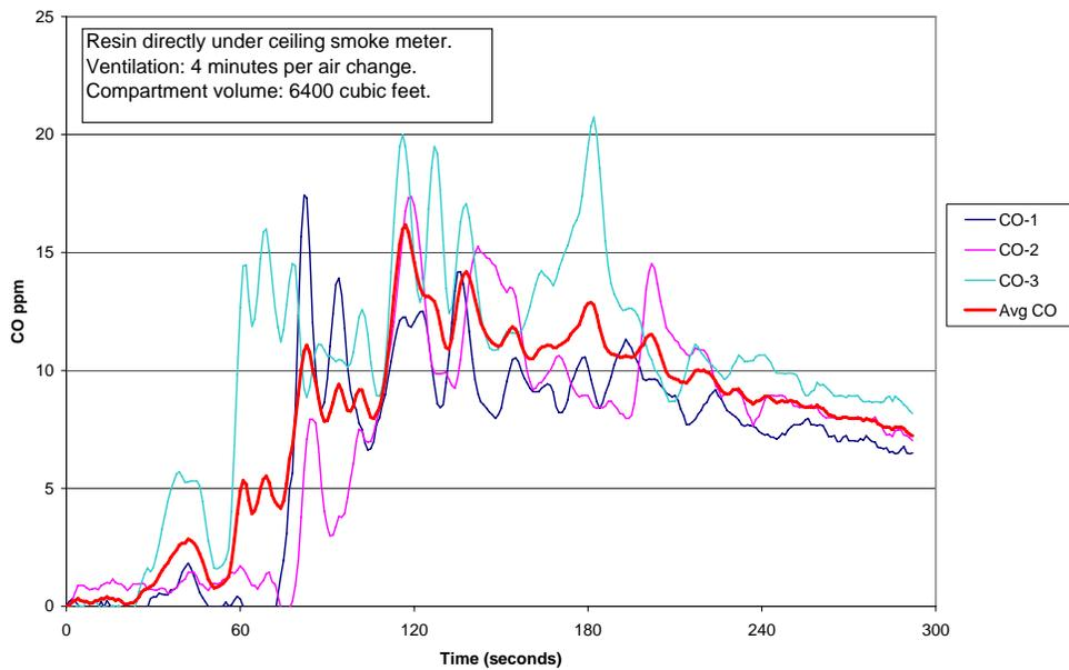
FIGURE 19. CO LEVELS IN THE DC-10 MAIN DECK COMPARTMENT
