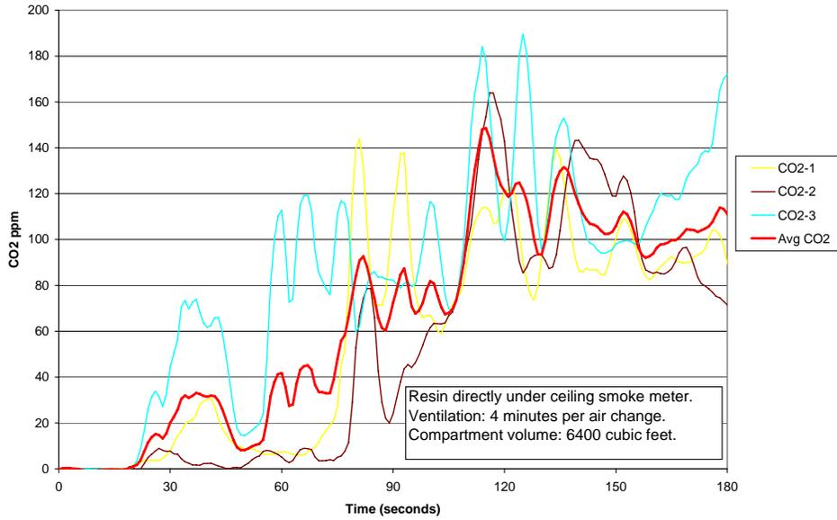
FIGURE 20. CO<sub>2</sub> LEVELS IN THE DC-10 MAIN DECK COMPARTMENT
