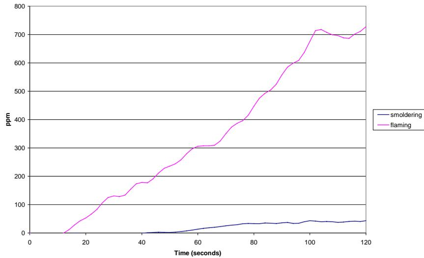
FIGURE 10. SMOLDERING AND FLAMING RESIN BLOCK CO<sub>2</sub> LEVELS NEAR THE CENTER OF COMPARTMENT
