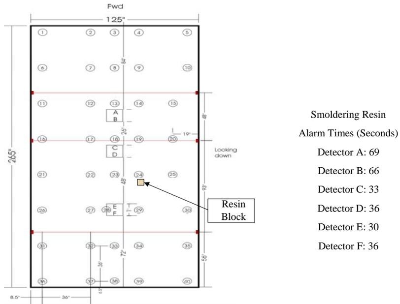
**FIGURE 4. SMOLDERING RESIN BLOCK NEAR THE CENTER OF B-707 CARGO COMPARTMENT**
