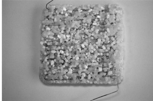
FIGURE 1. COMPRESSED PLASTIC RESIN BLOCK WITH IMBEDDED NICHROME WIRE
