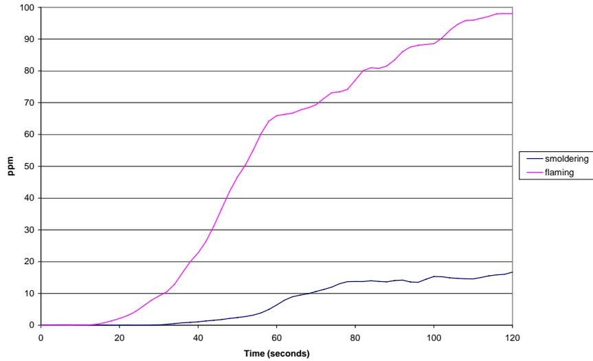
FIGURE 9. SMOLDERING AND FLAMING RESIN BLOCK CO LEVEL NEAR THE CENTER OF COMPARTMENT
