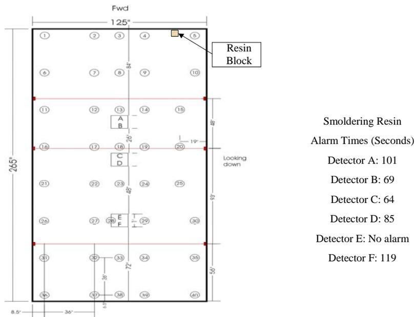
**FIGURE 5. SMOLDERING RESIN BLOCK IN THE FORWARD CORNER OF B-707 CARGO COMPARTMENT**
