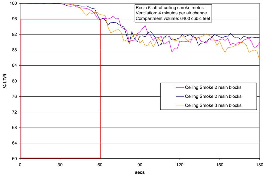
FIGURE 21. CEILING SMOKE LEVELS FROM MULTIPLE FLAMING RESIN BLOCKS IN THE DC-10 MAIN DECK COMPARTMENT
