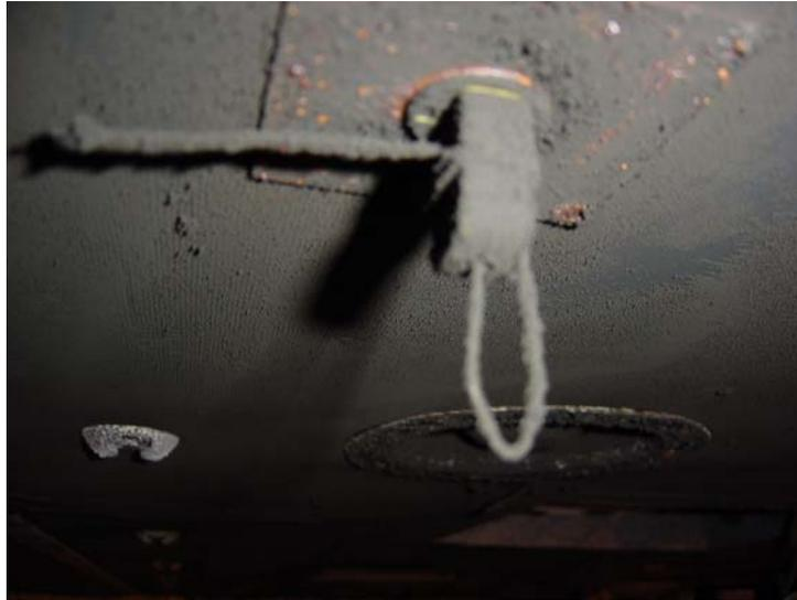
FIGURE 22. THERMOCOUPLE IN FULL-SCALE TEST FIXTURE
