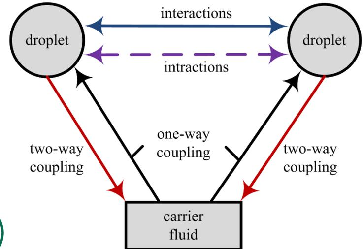
one-way: effect of carrier fluid on droplets
