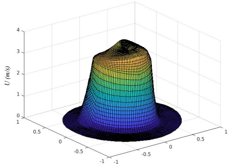
Inlet velocity profile reconstructed for simulation
