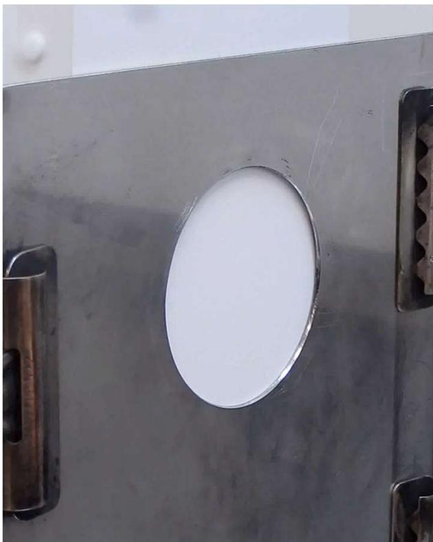
**Polystyrene Plate with 8 BL Clay/Polymer Coating (4 mm thick)**
