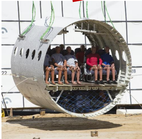
Vertical Impact test onto flat soil
