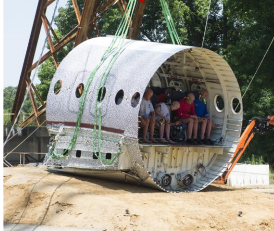
Canted vertical impact test onto sloped soil
