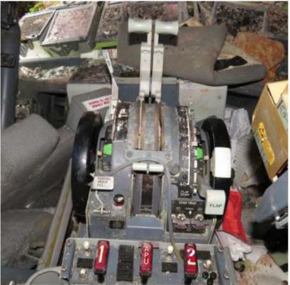
Control wheel and column on both sides were severely damaged. The rudder pedals were raised up and had jammed in the adjoining structure
