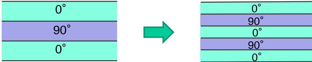
Propagation of the transverse crack is suppressed by constraining effect by neighboring layers.
