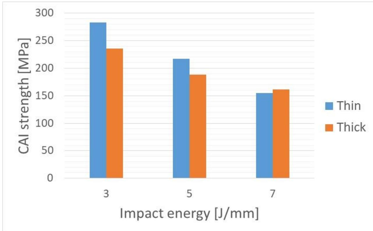
CAI strength was improved by decreasing ply thickness when the impact energy was below 5 J/mm. In contrast, reduction of CAI strength in thin ply laminates was confirmed when the impact energy was 7 J/mm.
