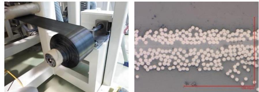
Picture and cross sectional image of thin ply thermoplastic prepreg
