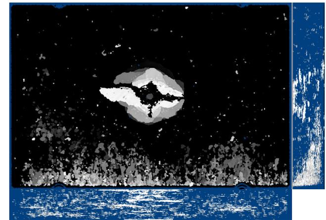
A large delamination at mid-plane that was typically seen in Thin ply laminates was suppressed by resin layer.
