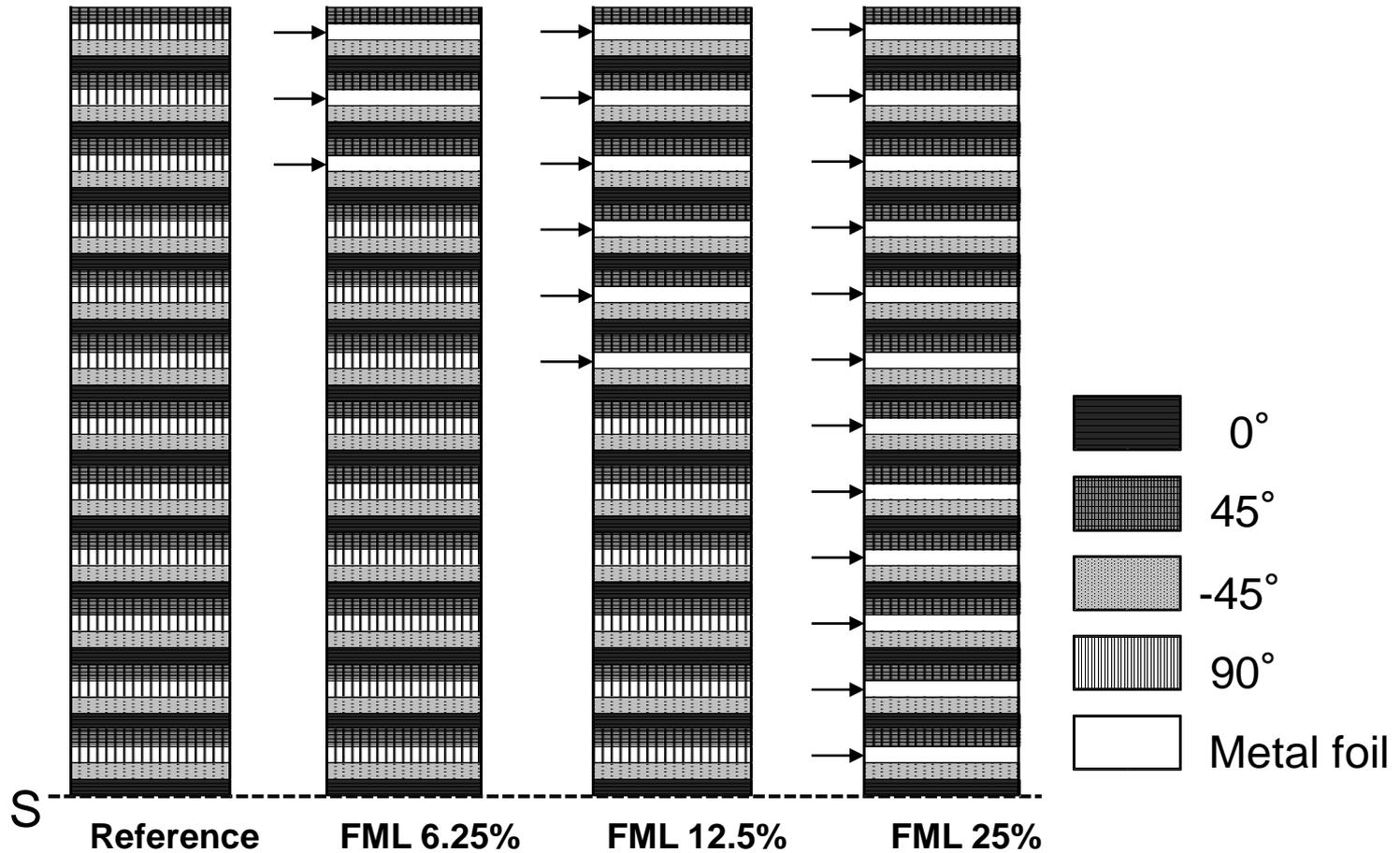
90° layers that hardly can bear the load were replaced to the metal foil (SUS301).
