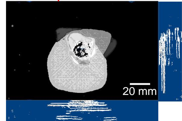
An extremely large delamination occurred near the mid-plane and the size of delamination became larger with increase of the impact energies. In addition, fiber breakage at the back face which deteriorated residual compressive strength was observed.
