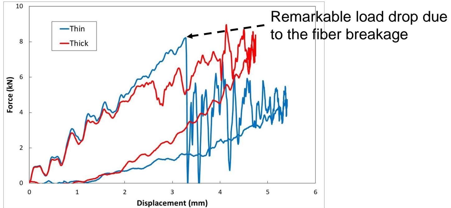
Force – displacement curves of the impact tests
