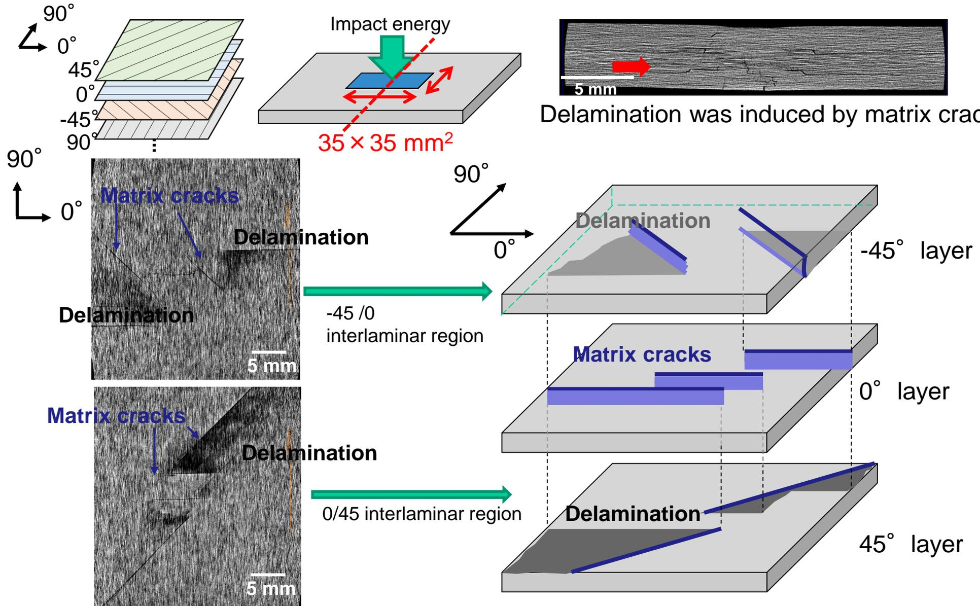
Matrix cracks occurred along the fiber direction in each layer and delamination occurred with connecting matrix cracks in neighbouring layers.
