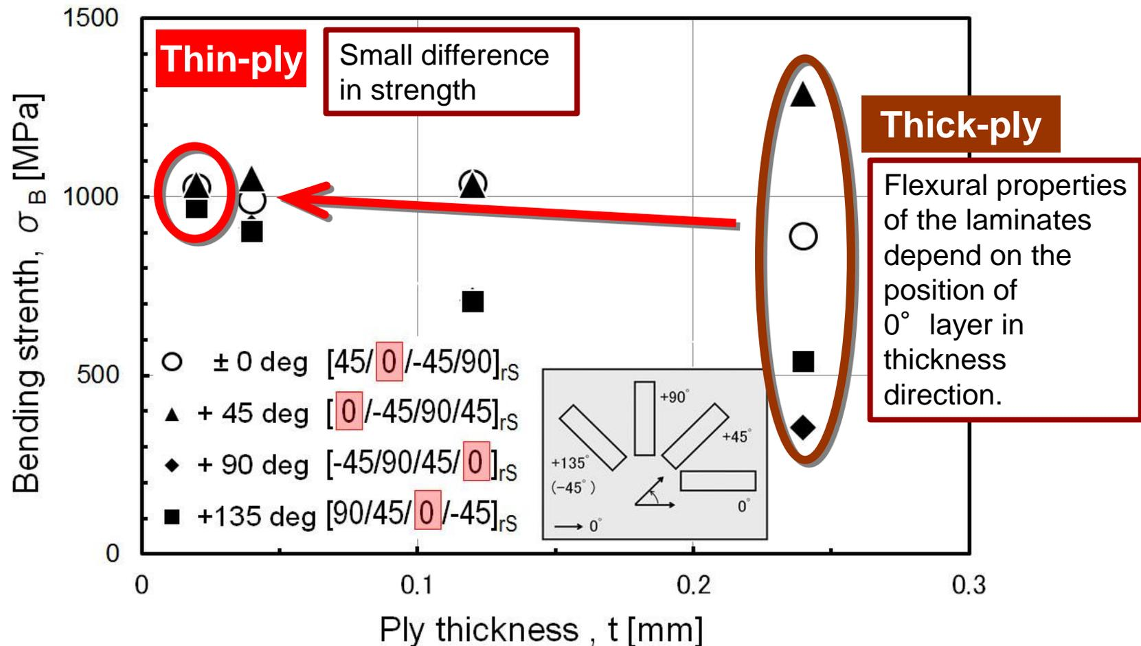
Differences in flexural properties between different directions were also decreased by decreasing ply thickness.
