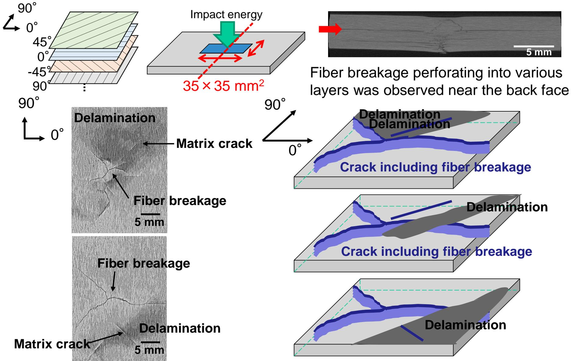
A large delamination near the mid-plane propagated with matrix cracks induced by fiber breakages.
