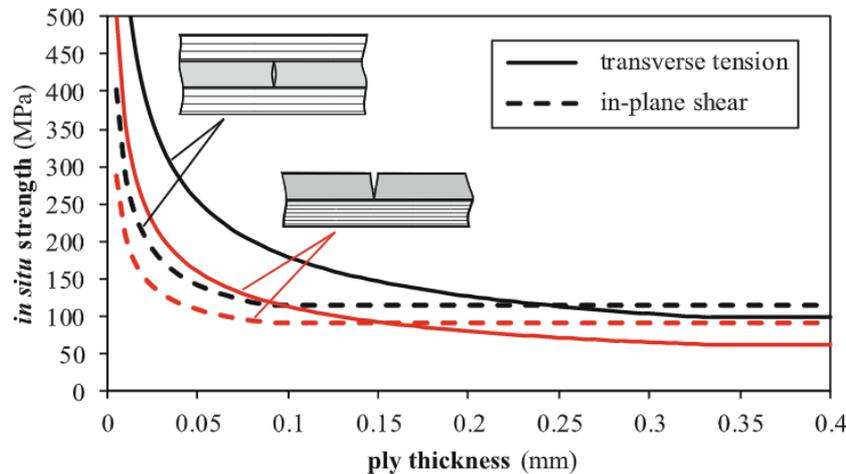
Relationship between in-situ strength and ply thickness [1]
