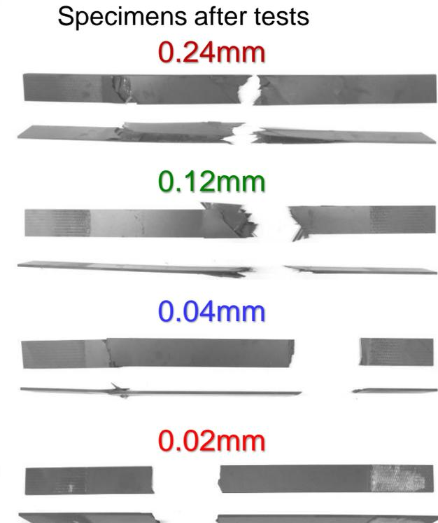
Delamination was suppressed until the final failure, thus tensile property was improved by decreasing ply thickness.
