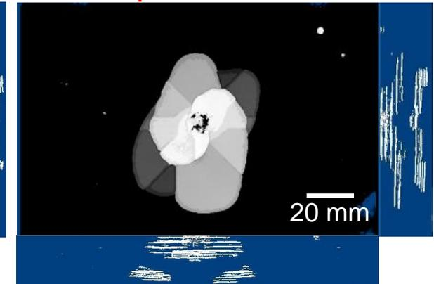
Distributed delaminations occurred in all interlaminar layers in thickness direction.
