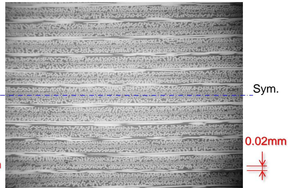
**The more ply can be inserted in case of thin ply laminates.**
