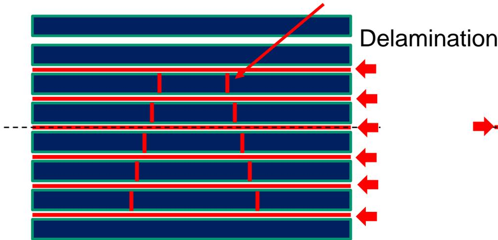
Matrix crack in each layer induced delamination.
