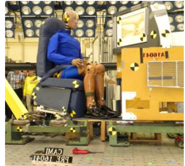
ATD with developmental lap-belt fitted airbag
