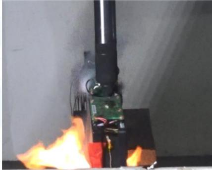
LFP nail penetration
