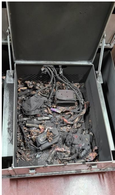
A4 Caught fire and exploded during overcharge test
