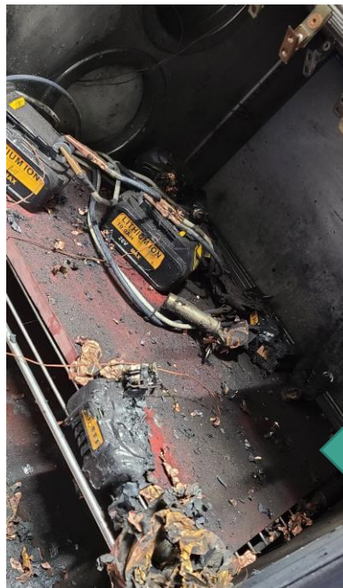
A4 Massive explosion during short- circuit test
