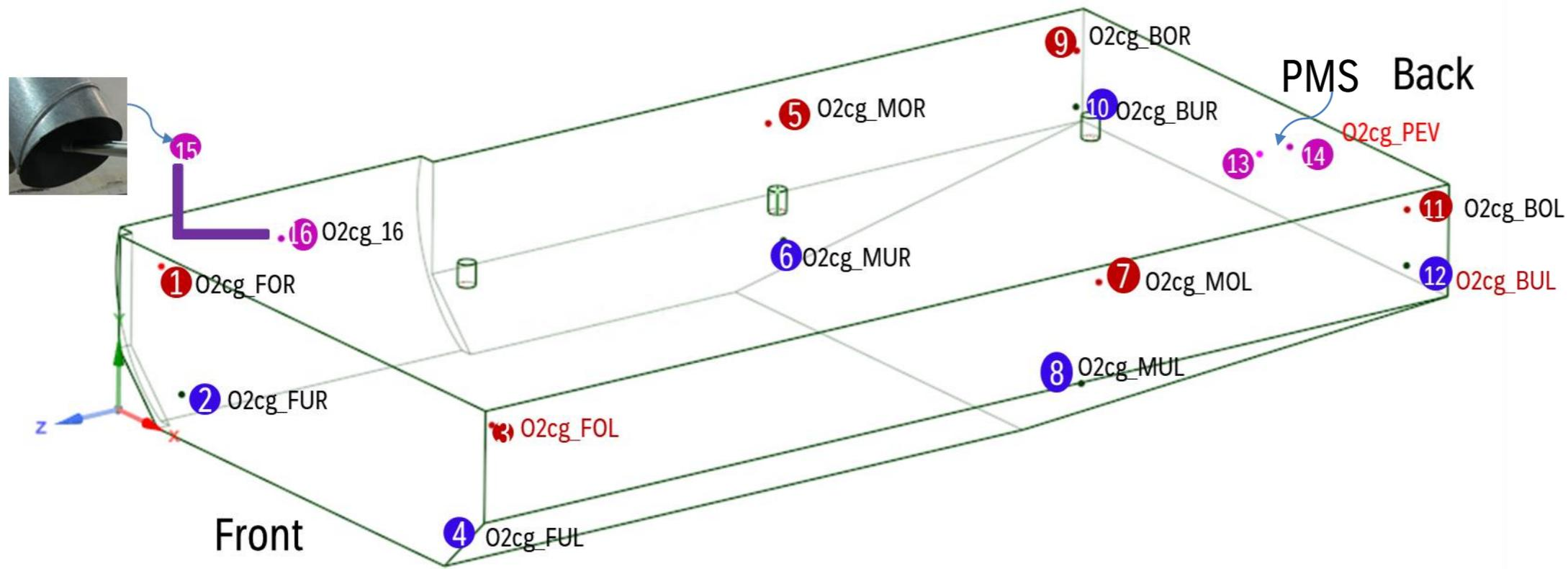
O<sub>2</sub> sensors are placed at 18 locations, near ceiling and floor, near side walls in between nozzles, in leakage pipe, near pressure management system (PMS)
