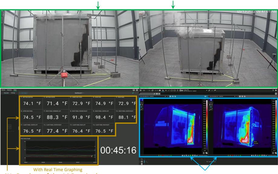
4Hz Readout of the 14 Required Thermocouples in AS8992
