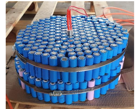
LIB bundle, worm-screw clamps and ignitor
