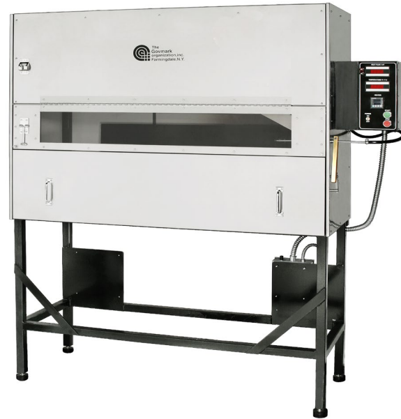
Radiant Panel (Thermo-acoustic Insulation) • Flame propagation distance • After flame time
