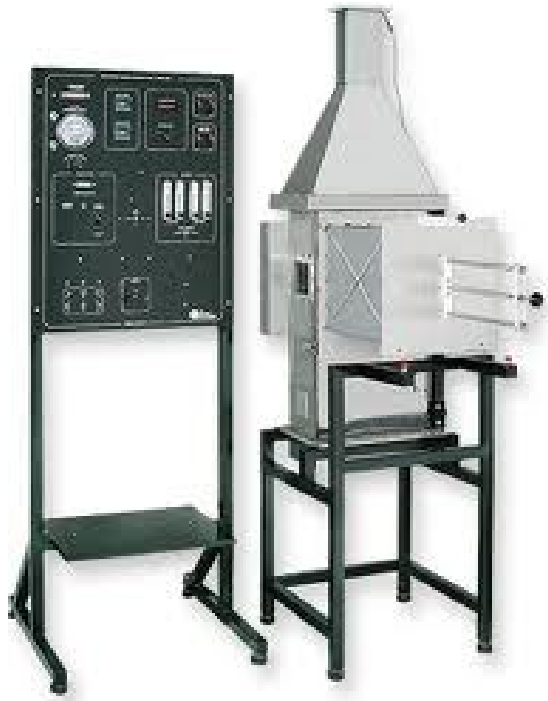
OSU Rate of Heat Release Apparatus (Large Area Materials) • Peak HRR • 2-min HR
