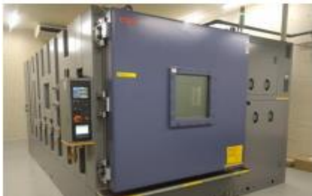
Temperature/Altitude/Humidity/ Icing Test Facility
