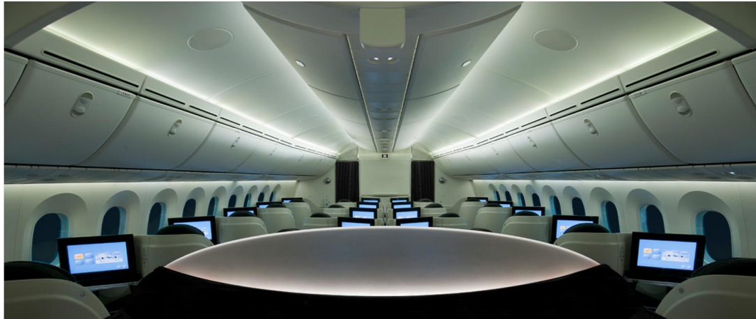
787 business class interior illustrating multiple large surfaces requiring heat release testing
