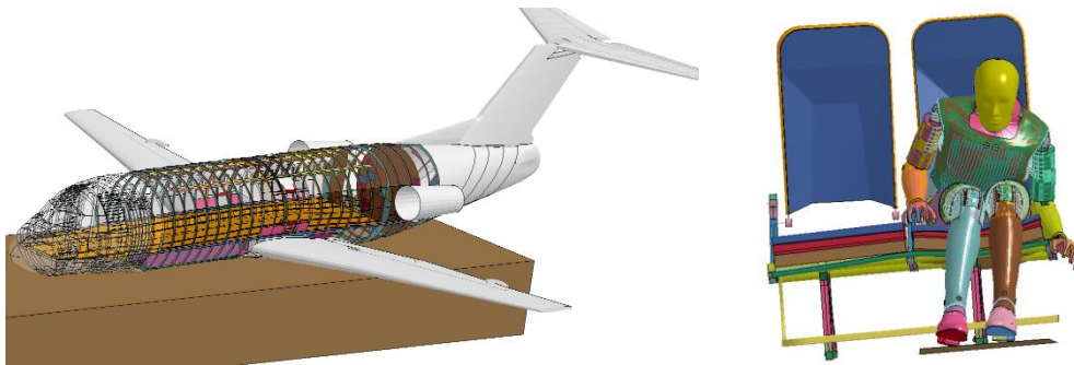
Figure 1. FE Simulation of the Fokker F28 (Left) and Occupant Breakout Model (Right)
