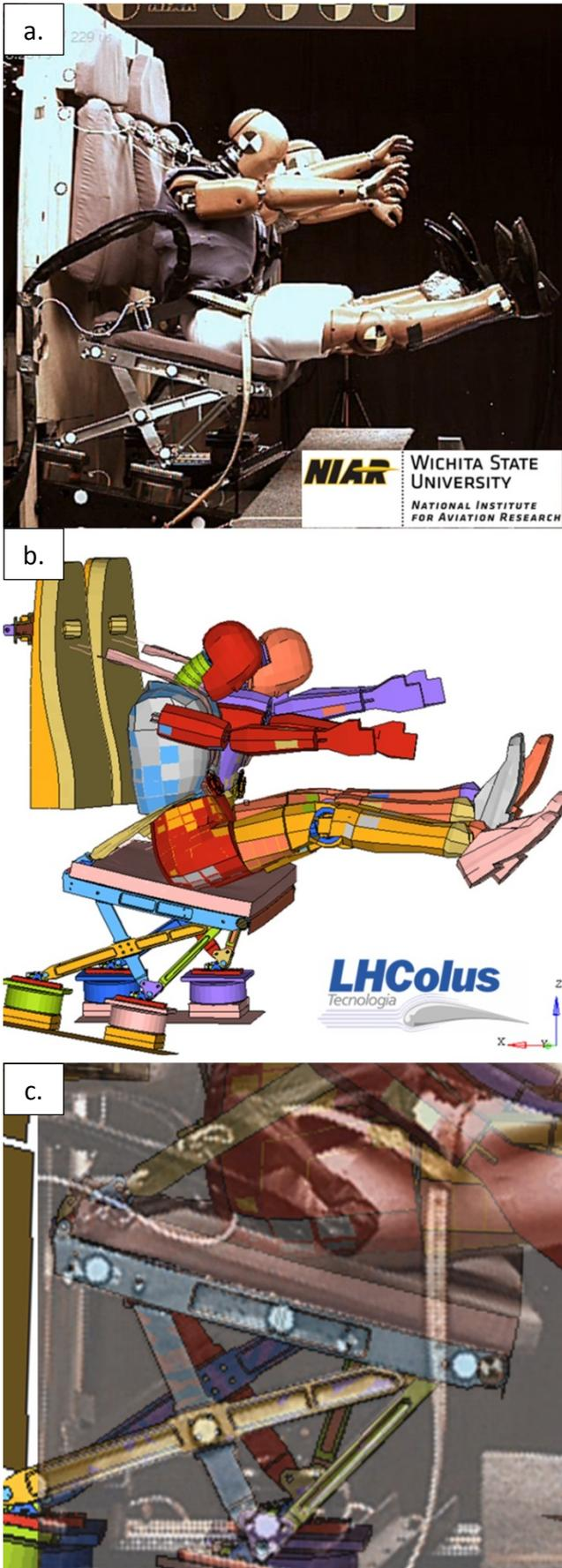
Figure 7 Comparison between analyses and test 16 FWD
