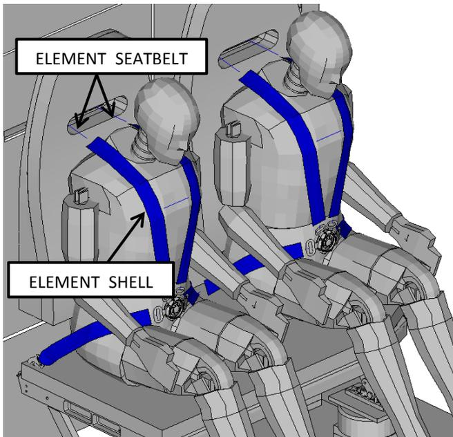
Figure 3 – Seatbelt Elements Analyses
