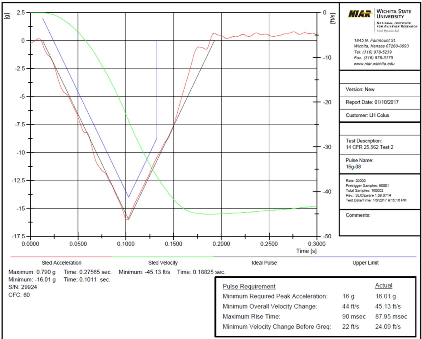
Figure 6 Acceleration and speed employed on the sled in the 16g FWD test
