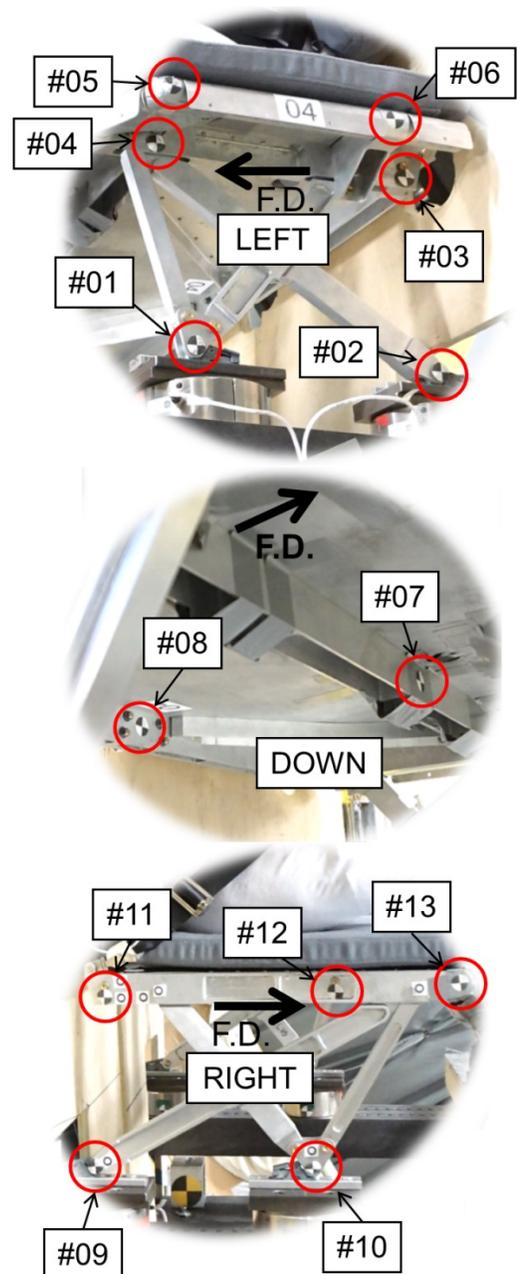
Figure 8 Measurement points of plastic deformation
