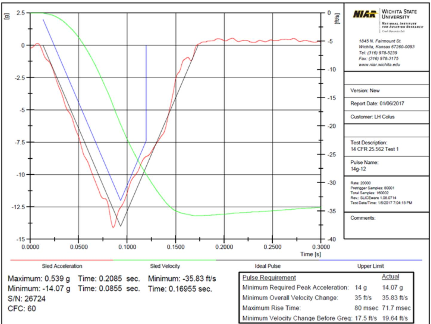
Figure 16 Acceleration and speed employed on the sled in the 14g DOWN test
