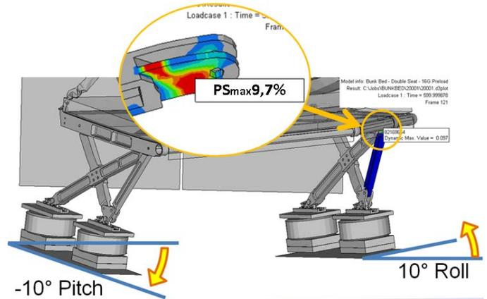
Figure 5 – Critical Case Evaluated in Dynamic Analyses
