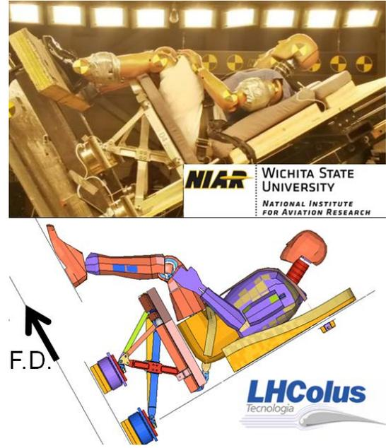
Figure 15 Test Setup 14g DOWN
