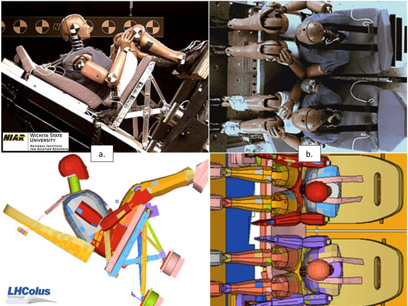
Figure 17 Kinematic behavior 14g DOWN
