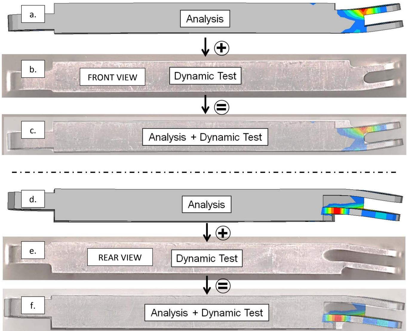
Figure 9 Maximum Plastic Strain Results
